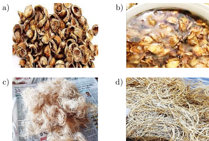
FIG. 2. Preparation of betel nut fiber: a) dry shell; b) moist shell; c) sun drying fiber; and d) processed fiber.
