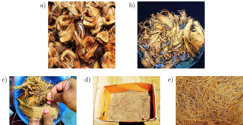
FIG. 1. Preparation of coir fiber: a) dry shell; b) moist shell; c) separate fiber from shell; d) sun drying fiber; and e) processed fiber.
