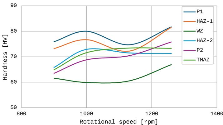
FIG. 8. Comparison of rotational speeds at various SZs.
