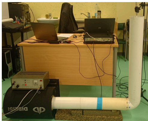
FIG. 8. View of experimental setup with an isolated sound source connected to a 1-meter long pipe with a diameter of 125 mm, including an acoustic helicoidal resonator at the end, a 90-degree elbow (typical in the ventilation market), and a 0.86-meter long outlet pipe oriented vertically (side up).
