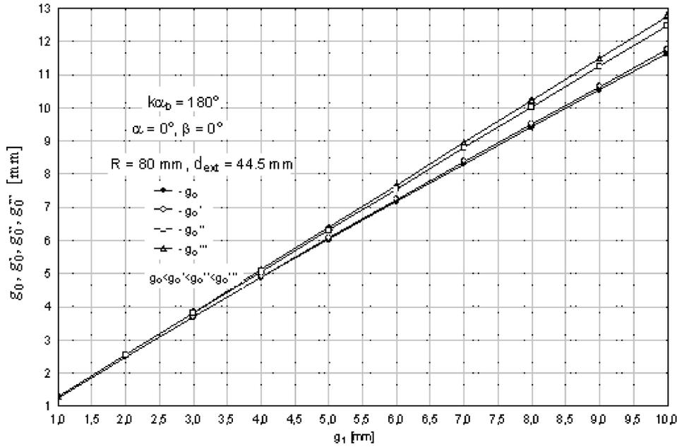
FIG. 3. Variation of the initial thickness of the tube wall depending on the calculated wall thickness  $g_1$  satisfying the conditions of the EU Standards [1] and UDT, see [12, 13].
