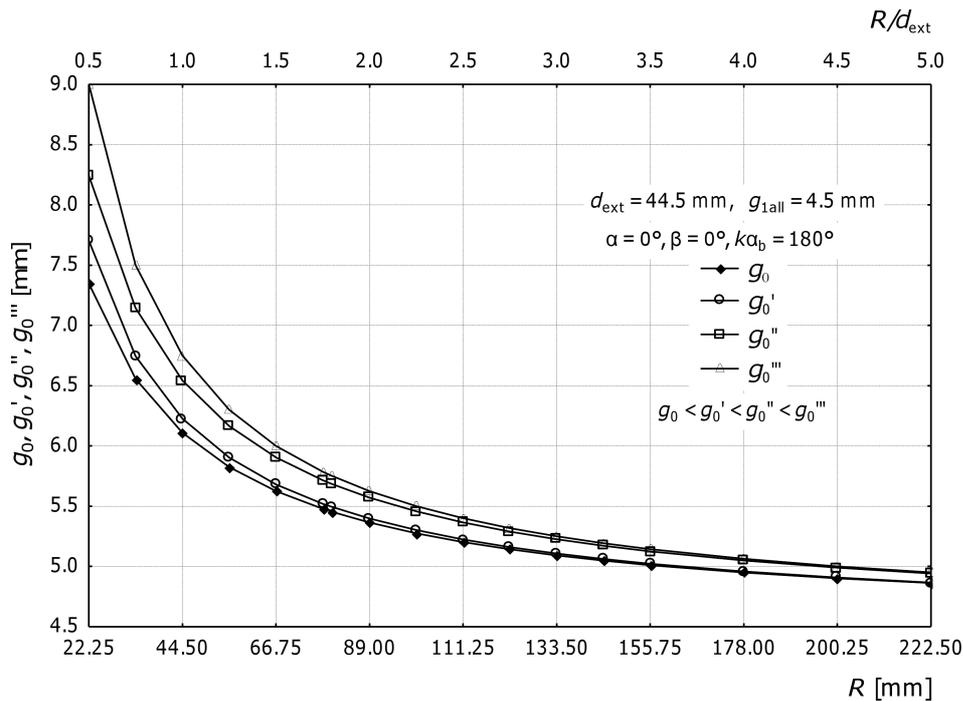
FIG. 2. Variation of the initial thickness versus  $R$  for four methods of calculations.
