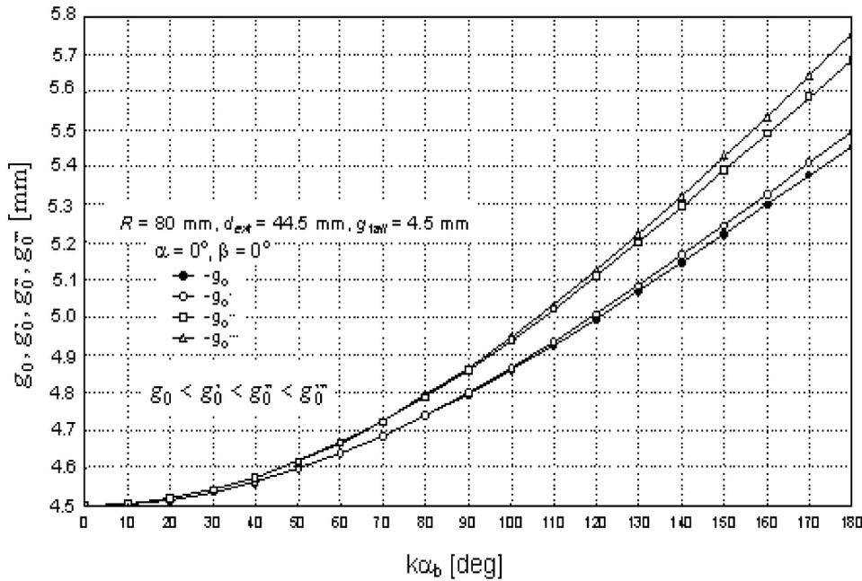
FIG. 1. Variation of the initial thickness versus  $k\alpha_b$  for four methods of calculations.
