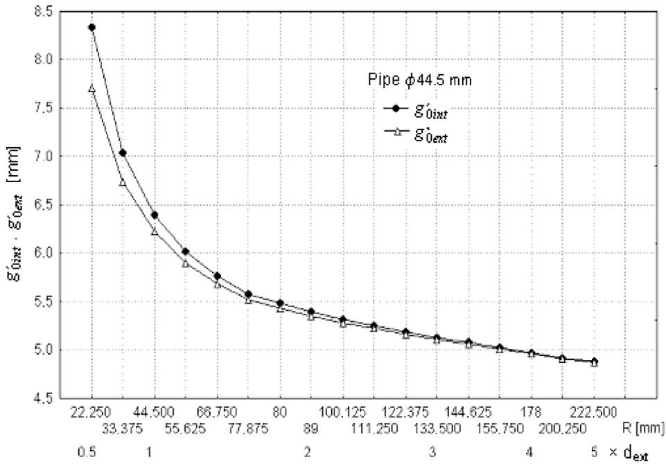
FIG. 4. Variation of the initial thickness ( $g'_{0ext}$ ,  $g'_{0int}$ ) of the wall of the tube for bending, calculated according to the simplification of the 1st order and in measures of logarithmic strains versus the bending radius  $R$ , when the required minimum wall thickness of the bent elbow is  $g_1 = 4.5$  mm.
