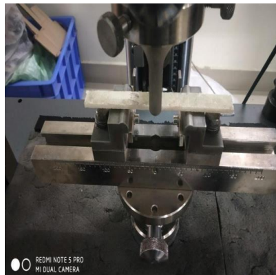
FIG. 5. Experimental setup for flexural test.
