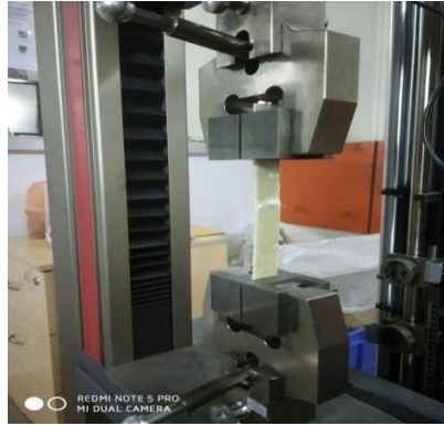
FIG. 3. Experimental setup for tensile test.
