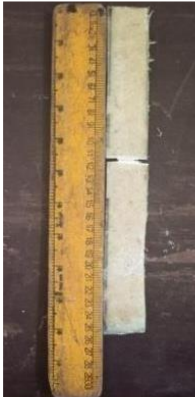
FIG. 4. Specimen after tensile testing.
