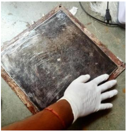
FIG. 1. Applying releasing agent.
