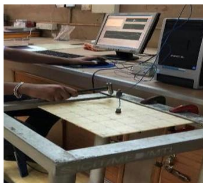
FIG. 6. Experimental setup for modal analysis.
