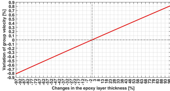
FIG. 26. The quantity  $\Delta V_G/V_G$  in relation to the variation in the epoxy layer thickness for the S0 mode at the frequency  $f = 10^{-3}$  MHz.
