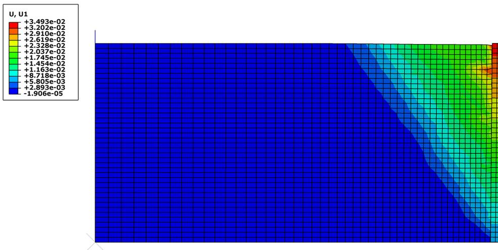
FIG. 4. Horizontal deformation for the incremental wall under a 70 kPa surcharge load.
