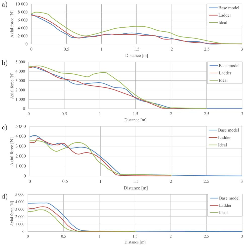
FIG. 12. Inductive forces of geogrids in three modes for full-height wall: a) geogrid layer 4, b) geogrid layer 3, c) geogrid layer 2, d) geogrid layer 1.
