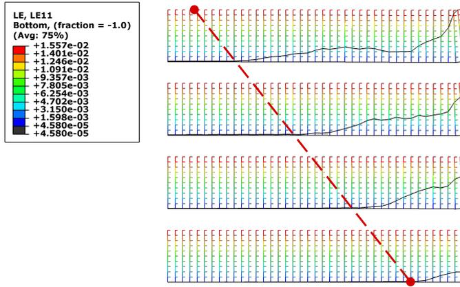
FIG. 9. Elastic strain induced in geogrid layers for the full-height wall.
