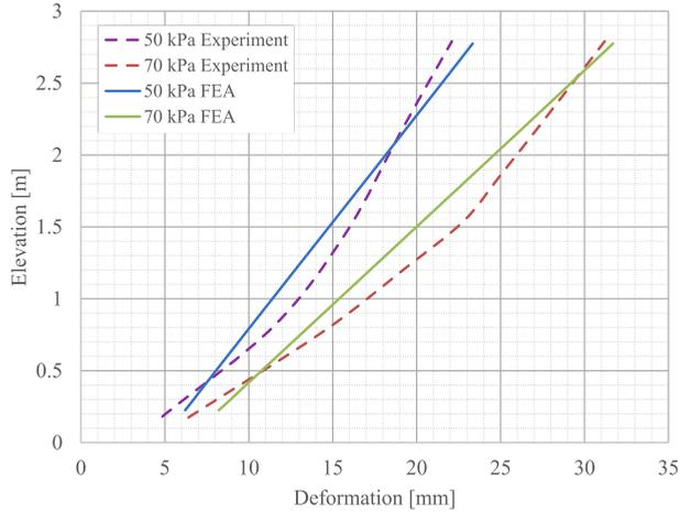
FIG. 5. The measured and modeled lateral deformation of the full-height panel wall.
