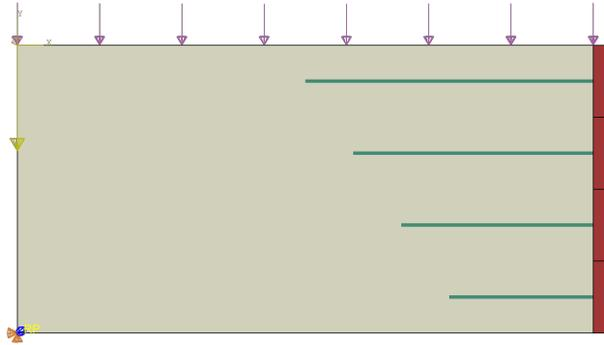
FIG. 11. The incremental wall model with reduced geogrid lengths (ladder mode).
