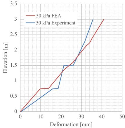
FIG. 6. The measured and modeled lateral deformation of the incremental wall.
