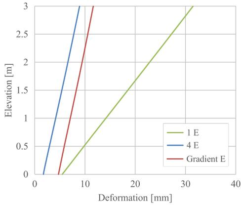
FIG. 7. The full-height wall displacement for different layer stiffness.
