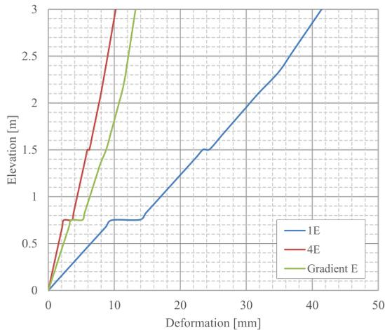
FIG. 8. The incremental wall displacement for different layer stiffness.
