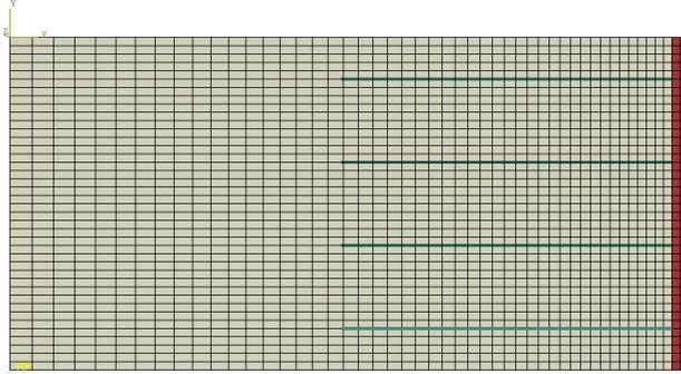
FIG. 3. FE Mesh of the model.
