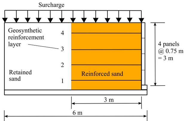
FIG. 1. The geometry of GRS walls constructed at RMCC [3].
