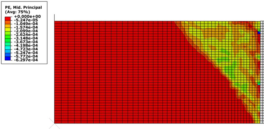
FIG. 10. Average plastic strains in the soil for the full-height wall.
