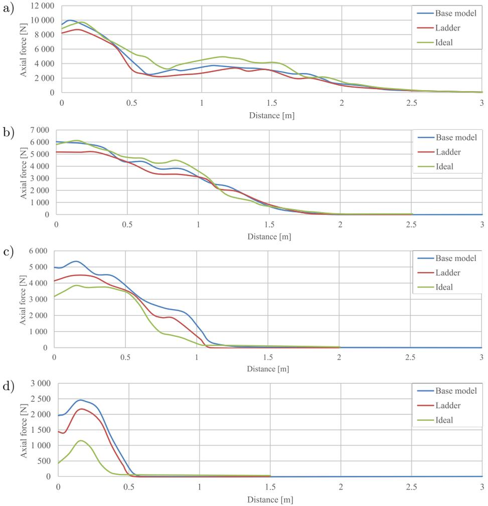
FIG. 13. Inductive forces of geogrids in three modes for incremental wall:
