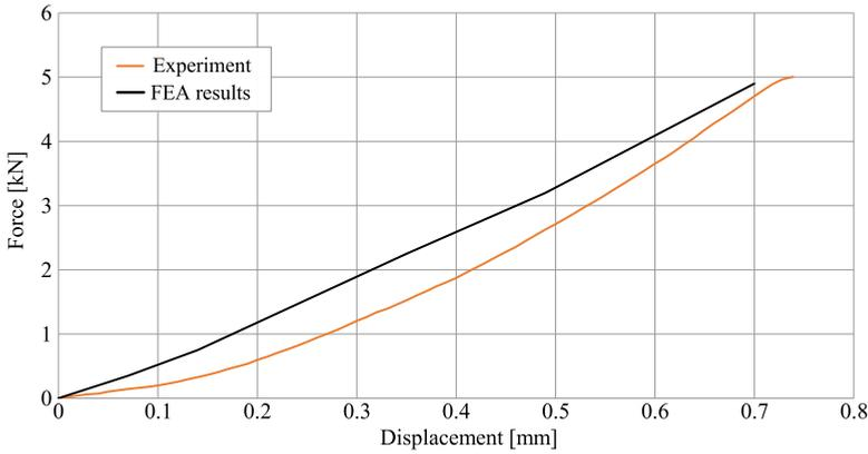
FIG. 10. Comparison of experiment results and FEA simulation results in the range of 0 to 0.7 mm.
