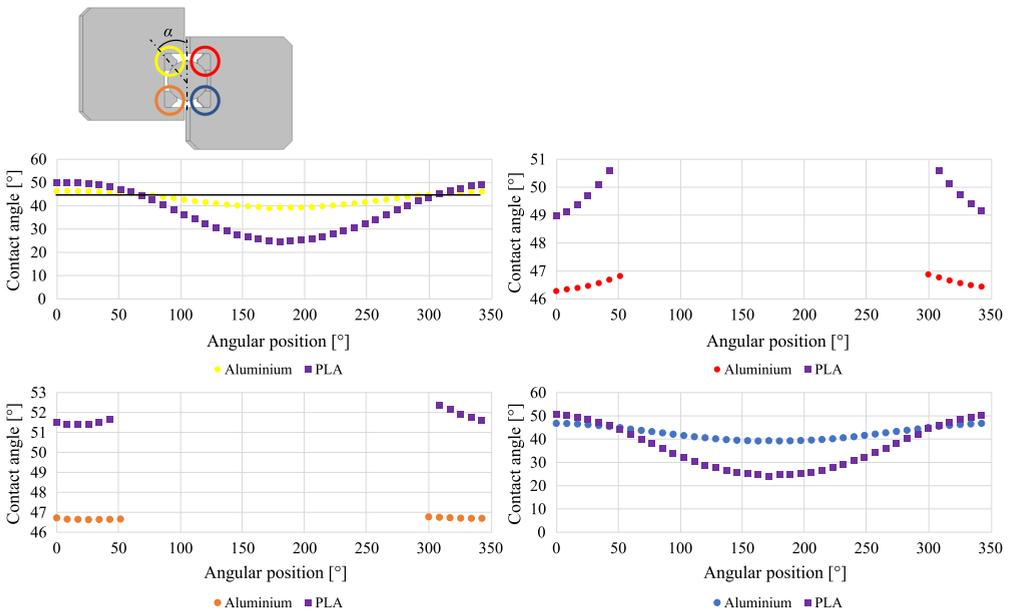
**FIG. 12.** Comparison of contact angle for every contact pair in wire raceway bearing.
