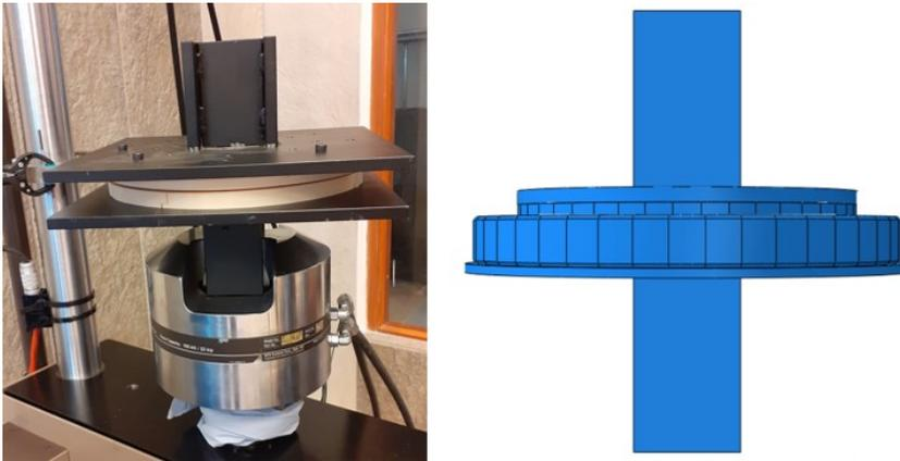
FIG. 8. The assembly of the test jig and the prototype of 3D printed wire raceway bearing (left side) and the FEA equivalent model with the test jig used in the simulation (right side).
