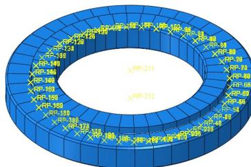
FIG. 7. An example of the FEA equivalent model of wire raceway bearing.
