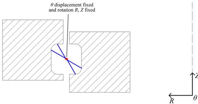
FIG. 6. Boundary conditions for sets of spring and beam elements (only 2 spring and beam elements were presented for clarity).
