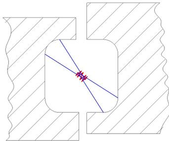
FIG. 3. The concept of the FEA equivalent model (red color – spring elements, blue color – rigid beam elements) shown only for two contact pairs.
