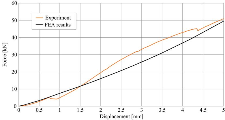
FIG. 9. Comparison of experiment results and FEA simulation results.
