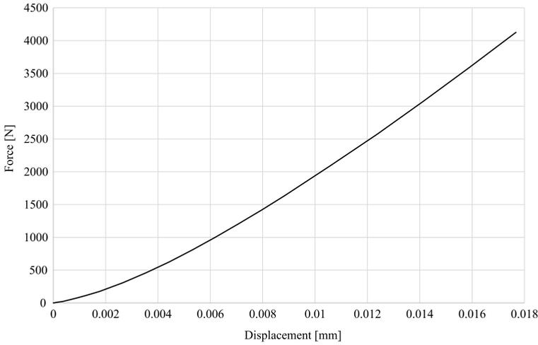
FIG. 4. Nonlinear spring stiffness used in the FEA equivalent model.
