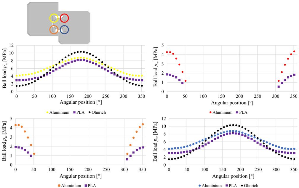
FIG. 11. Comparison of ball load for every contact pair in wire raceway bearing.
