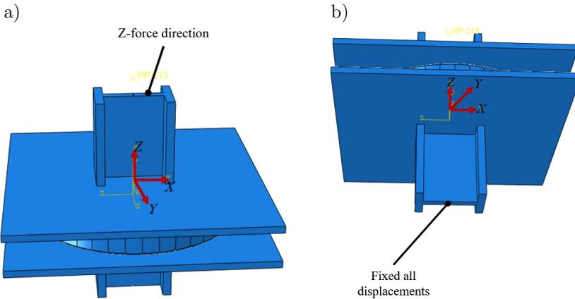
FIG. 5. Boundary conditions used in FEA: a) the upper part of the test jig, b) the bottom part of the test jig.
