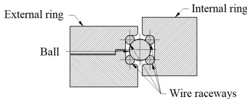
FIG. 1. The section view of the wire raceway bearing.
