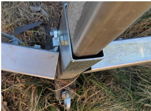
FIG. 8. Bending of the frame beam connectors.
