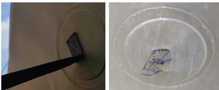
FIG. 9. The connections of the frame with the tent canopy: before the hurricane (left) and after the hurricane (right).
