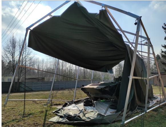
FIG. 6. Failure of the tent due to prolonged exposure to a hurricane.
