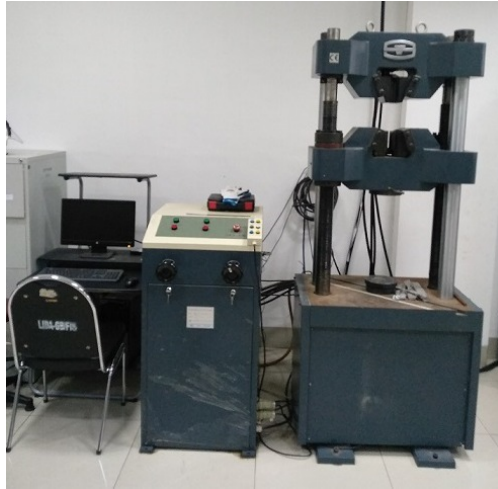
FIG. 2. The testing machine of UTM.
