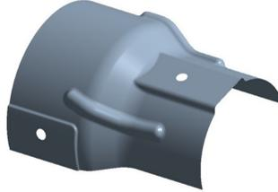
FIG. 3. Geometrical model of the muffler shield.
