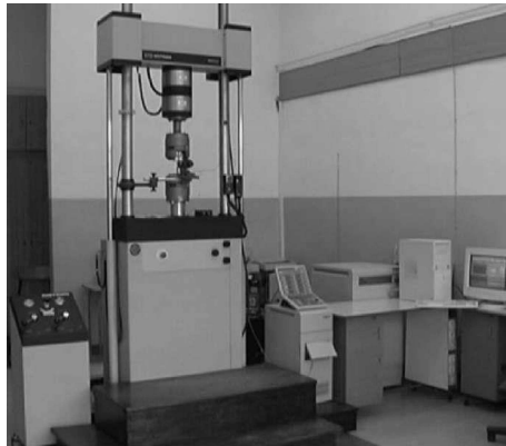
FIG. 3. Crushing strength measuring station with an INSTRON-8502 servo-hydraulic frame.
