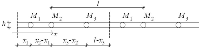
FIG. 1. The plate strip with a system of three periodically distributed concentrated masses.
