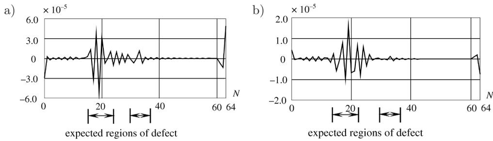
FIG. 19. DWT (Daubechies 4, detail 1) signal: curvature  $\kappa_x$  (a) and  $\kappa_y$  (b) measured at point D,  $N$  – number of measurements.
