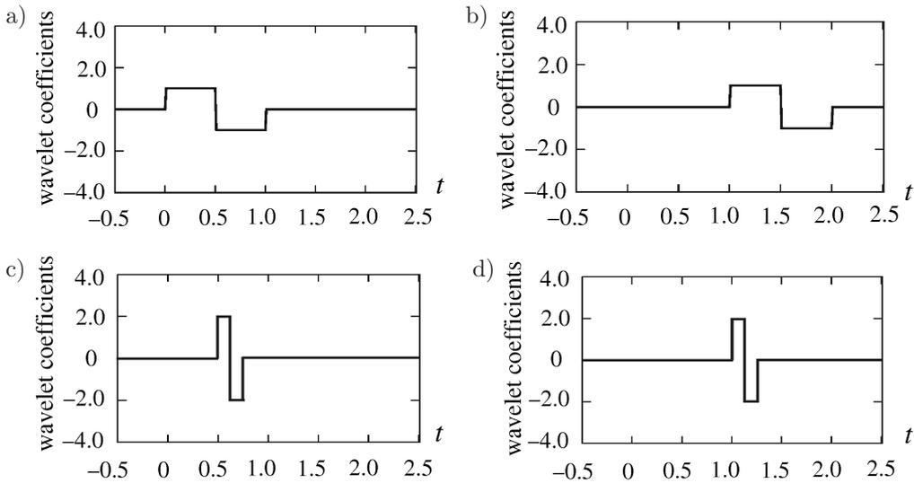
FIG. 1. Haar wavelet family: a) mother wavelet  $j = 0, k = 0$ , b) wavelet with parameters  $j = 0, k = 1$ , c)  $j = 2, k = 2$ , d)  $j = 2, k = 4$ .
