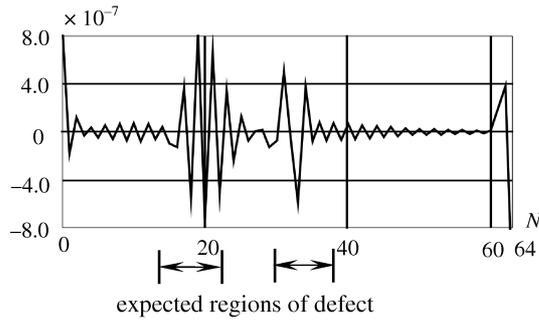
FIG. 18. DWT (Daubechies 4, detail 1) signal: vertical displacements measured at point D,  $N$  – number of measurements.
