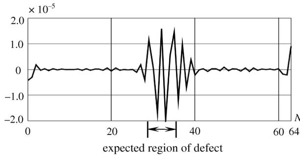
FIG. 21. DWT (Daubechies 4, detail 1) signal: amplitudes of the vertical displacements measured at point D,  $N$  – number of measurements.
