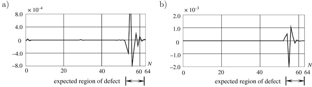
FIG. 16. DWT (Daubechies4, detail 1) signal: curvature  $\kappa_x$  (a) and  $\kappa_y$  (b) measured at point D,  $N$  – number of measurements.
