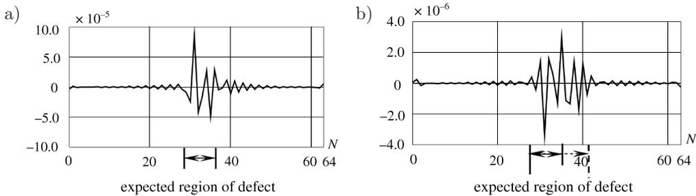
FIG. 7. DWT (Daubechies 4, detail 1) signal: curvature  $\kappa_x$  (a) and  $\kappa_y$  (b) measured at point D,  $N$  – number of measurements.
