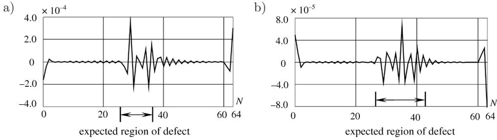
FIG. 13. DWT (Daubechies 4, detail 1) signal: curvature  $\kappa_x$  (a) and  $\kappa_y$  (b) measured at point D,  $N$  – number of measurements.
