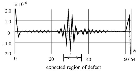
FIG. 9. DWT (Daubechies 4, detail 1) signal: vertical displacements measured at point D,  $N$  – number of measurements.
