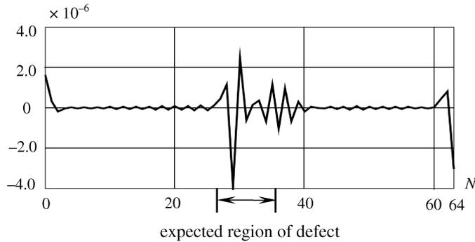
FIG. 12. DWT (Daubechies 4, detail 1) signal: vertical displacements measured at point D,  $N$  – number of measurements.
