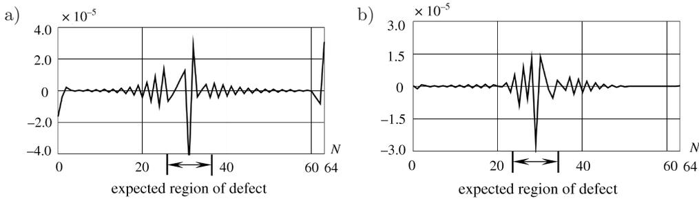
FIG. 10. DWT (Daubechies 4, detail 1) signal: curvature  $\kappa_x$  (a) and  $\kappa_y$  (b) measured at the point D,  $N$  – number of measurements.
