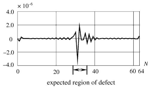
FIG. 6. DWT (Daubechies 4, detail 1) signal: vertical displacements measured at point D  $N$  – number of measurements.
