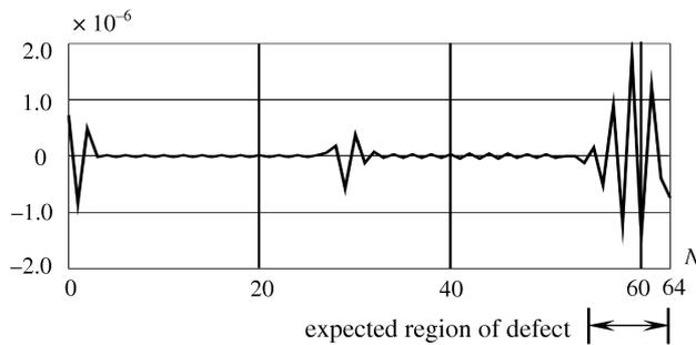
FIG. 15. DWT (Daubechies 4, detail 1) signal: vertical displacements measured at point D,  $N$  – number of measurements.
