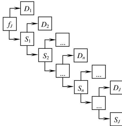
FIG. 2. Mallat pyramid algorithm [13].
