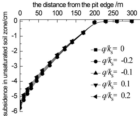
FIG. 8. Effect of initial suction on settlement in the unsaturated zone.
