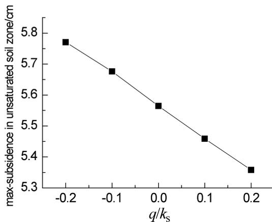
FIG. 9. Relationship between initial suction and maximum settlement in the unsaturated zone.
