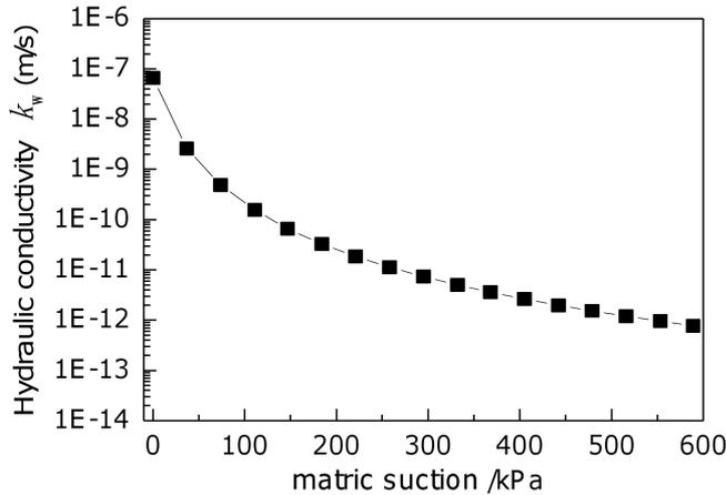
FIG. 5. Hydraulic conductivity for unsaturated soil.
