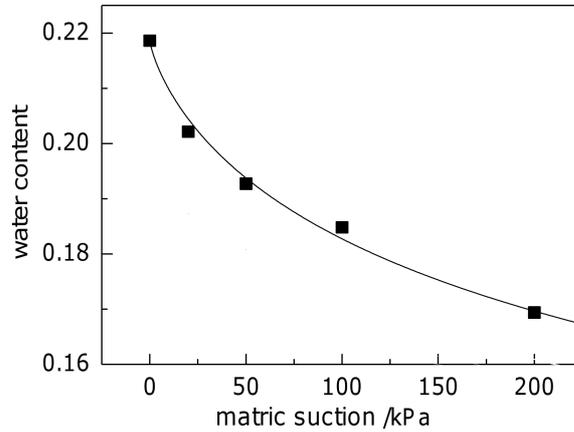
FIG. 3. The soil-water characteristic curve.
