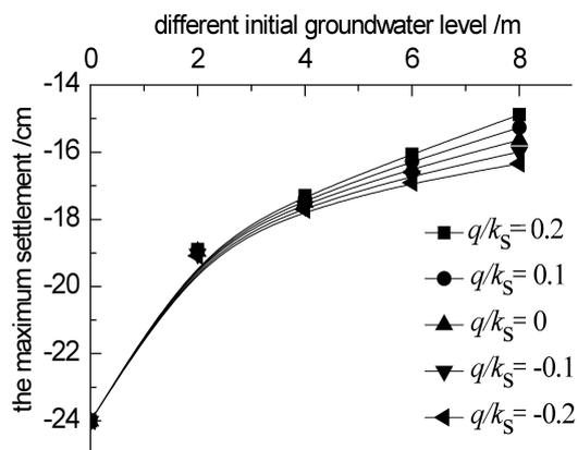
FIG. 12. Effect of  $q/k_s$  on total settlement at different initial water tables.
