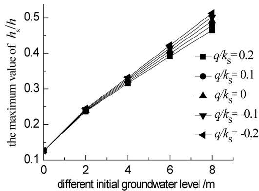
FIG. 13. Effect of  $q/k_s$  on  $h_s/h$  at different initial water tables.
