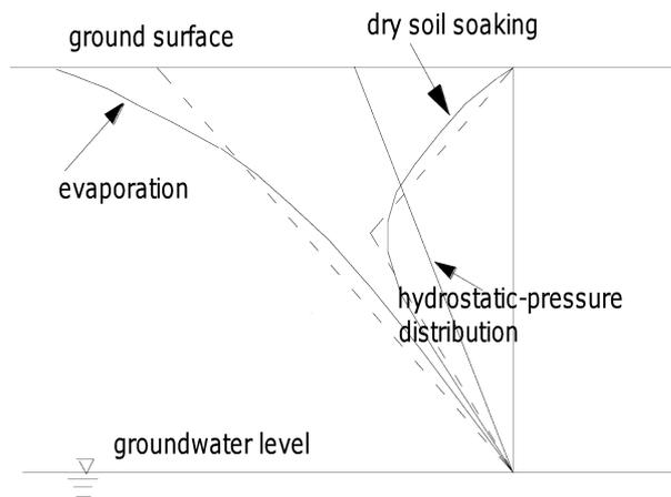
FIG. 1. Distribution pattern of matric suction along the depth of slope from ground surface.
