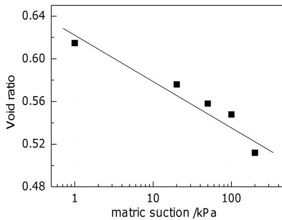
FIG. 4. Relationship between matric suction and void ratio.
