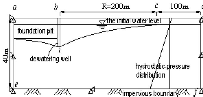
FIG. 2. Sketch of foundation pit dewatering.
