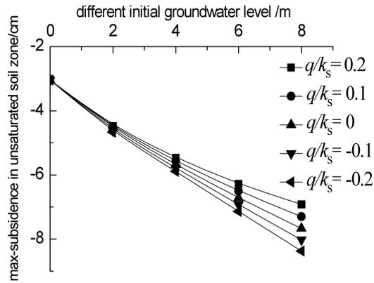
FIG. 11. Effect of  $q/k_s$  on settlement in unsaturated zone at different initial water tables.
