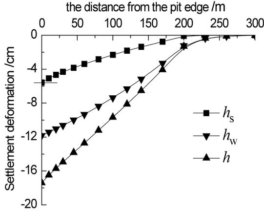
FIG. 6. Analysis of settlement curve.
