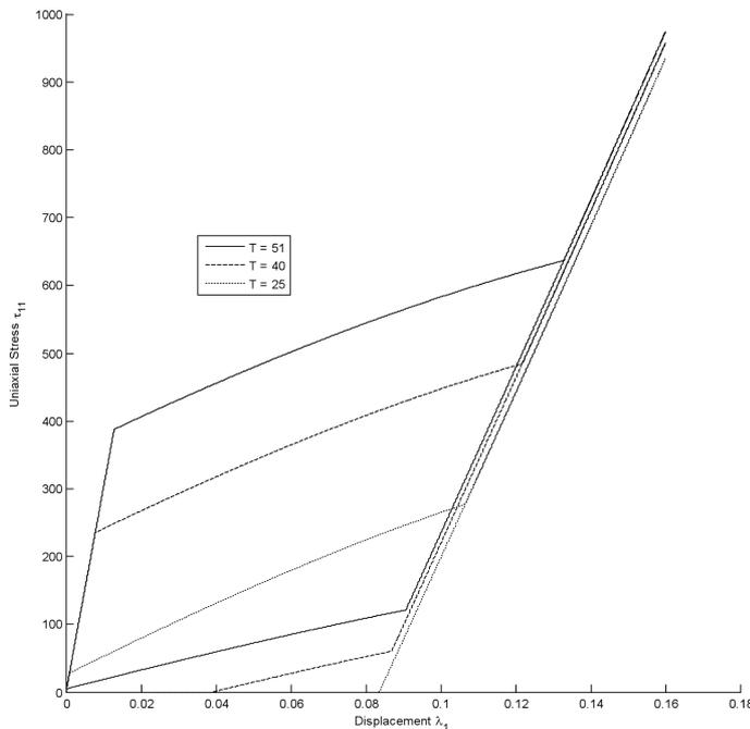
FIG. 2. Uniaxial tension. Uniaxial stress  $\tau_{11}$  vs. axial strain  $\lambda_1$  for different values of the (reference) temperature  $T$ .
