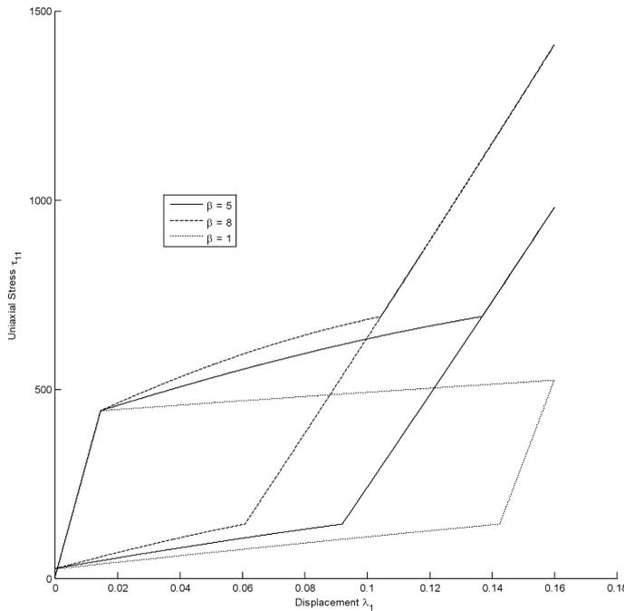
FIG. 1. Uniaxial tension. Uniaxial stress  $\tau_{11}$  vs. axial strain  $\lambda_1$  for different values of  $\beta$ .
