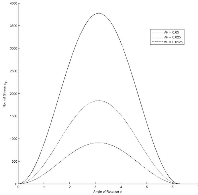
FIG. 4. Cycle 1: Normal stress  $\tau_{11}$  vs. angle of rotation  $\phi$ .
