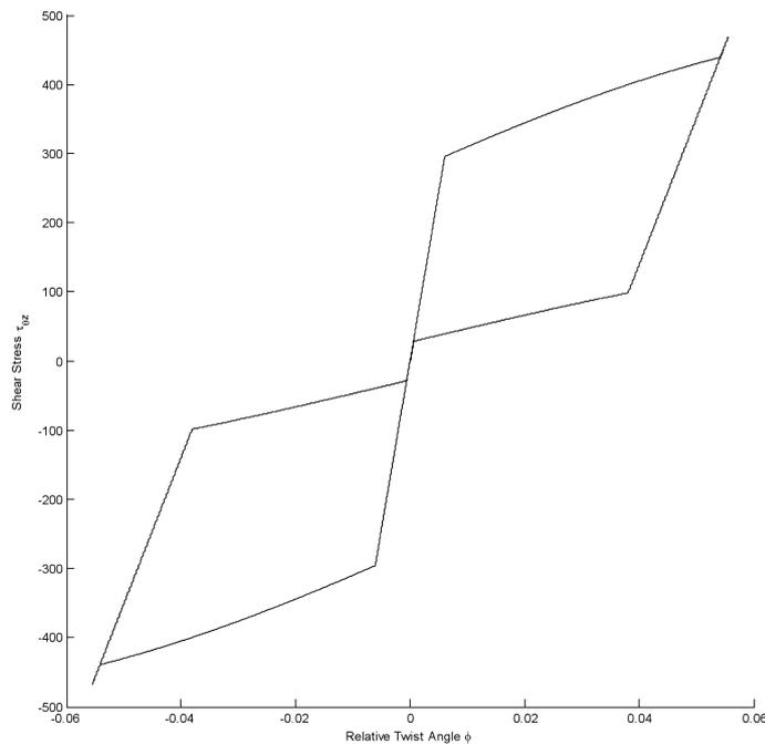
FIG. 3. Torsion of an SMA tube: Shear stress  $\tau_{\theta z}$  vs. relative angle of twist  $\phi$ .
