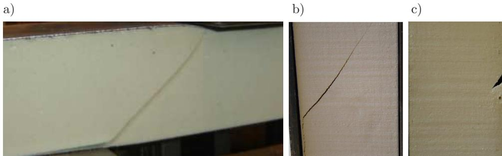
FIG. 2. Cracks obtained during: a) four point bending test, b), c) double lap shear test.
