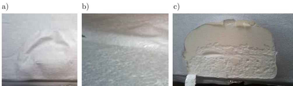
FIG. 3. a) blister, b) blister with damaged face sheet, c) visible core after removing the blister.
