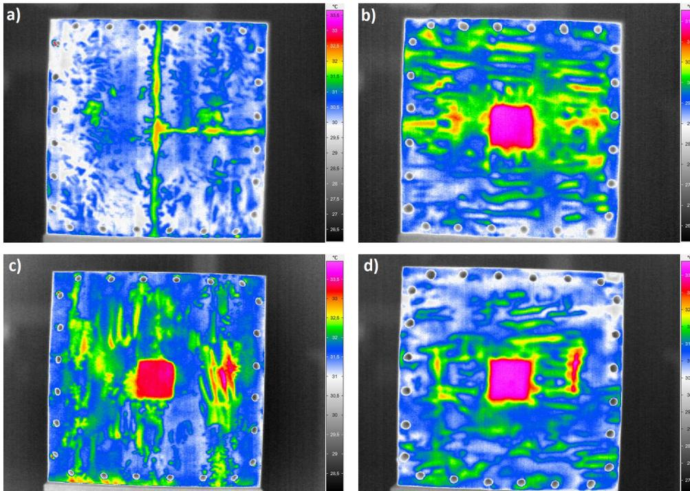
FIG. 6. Thermograms for a) cracked core, b) 1/2 local lack of a core, c) 1/4 local lack of a core, d) local lacks of an adhesive.
