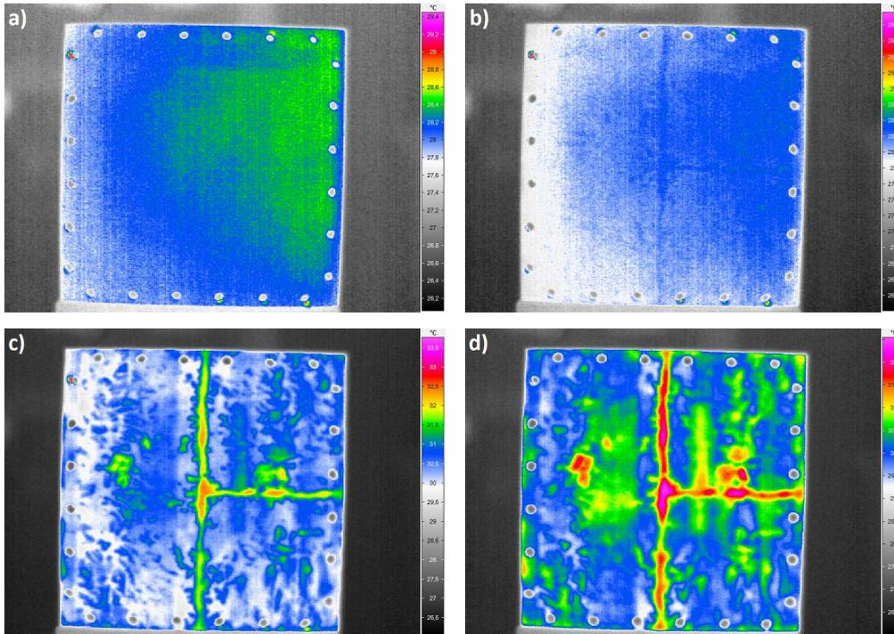
FIG. 5. Exemplary thermograms obtained during the experiment: a) before excitation, b) during excitation, c) 4 s after excitation, d) 10 s after excitation.
