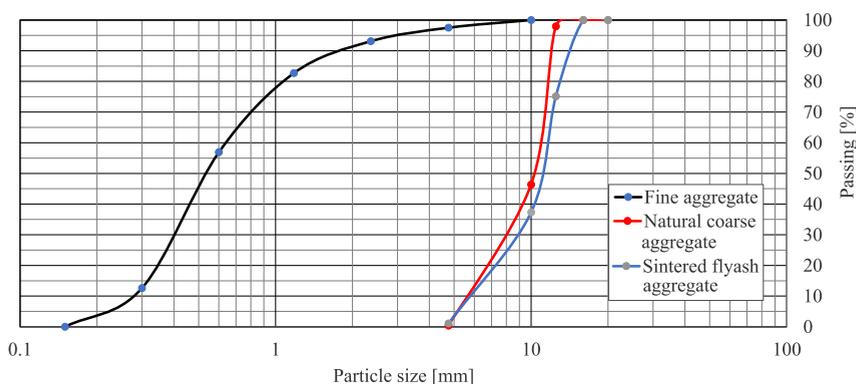
FIG. 2. Particle size distribution curve for fine aggregate, natural coarse aggregate and sintered fly ash aggregate.
