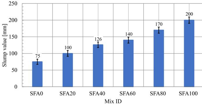
FIG. 3. Various levels of slump values for different percentages of SFA.
