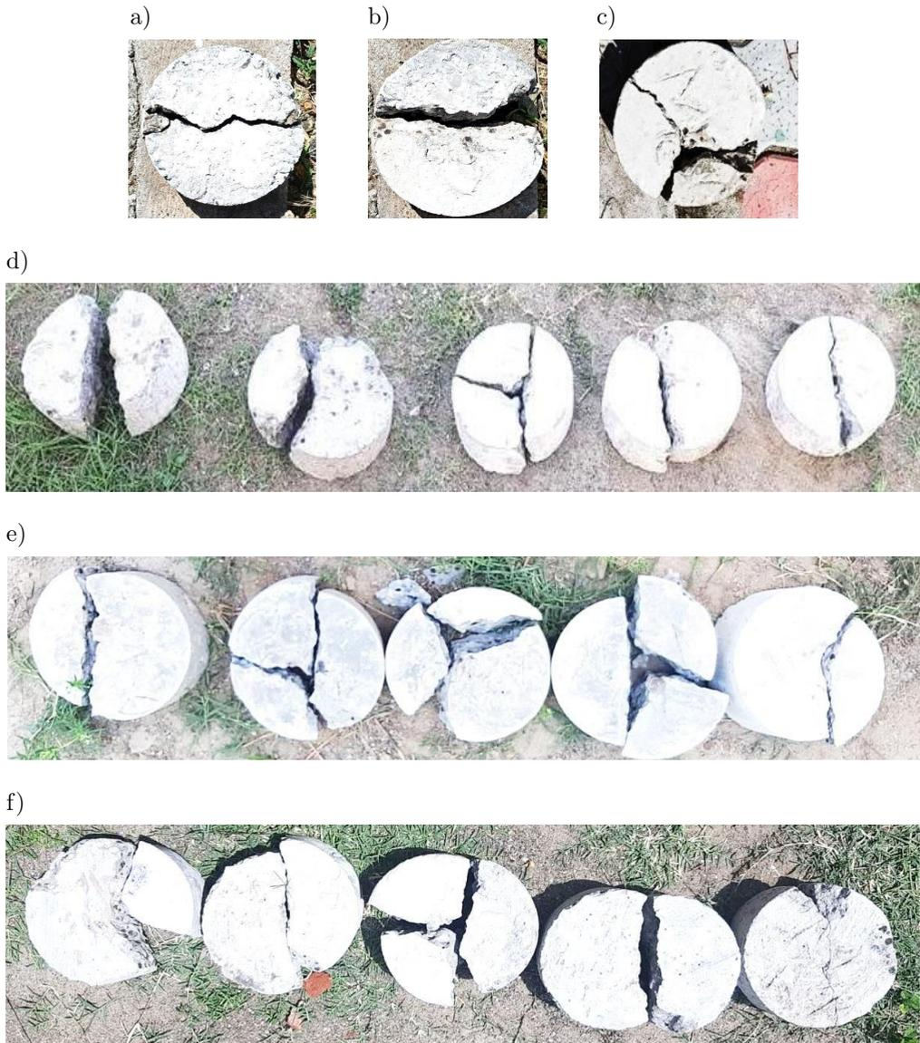
FIG. 10. Failure specimens for the typical concrete mix:
