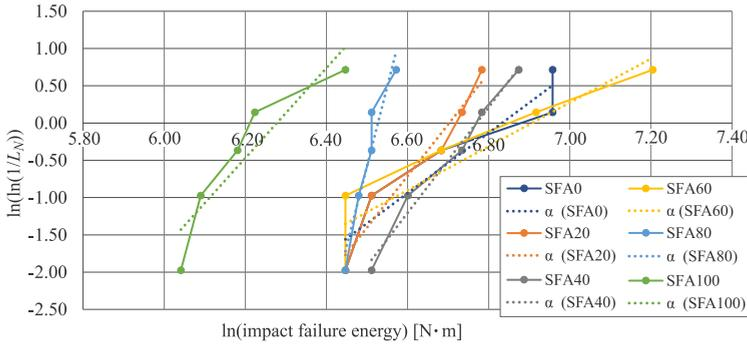
FIG. 11. Linear regression analysis based on the Weibull distribution for the percentage of varying SFA.
