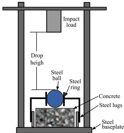
FIG. 8. A typical view of drop weight impact test [25].
