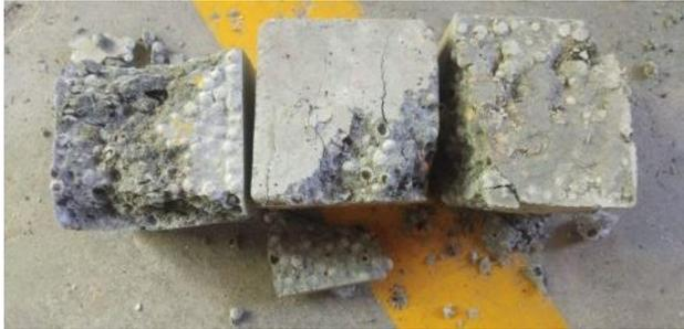
FIG. 7. Typical failure of concrete cubes for concrete mixture SFA 100.
