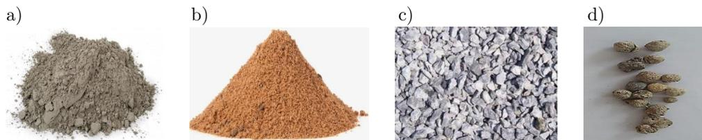
FIG. 1. Concrete material ingredients: a) cement, b) fine aggregate, c) NCA, d) SFA.
