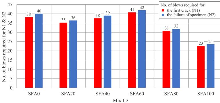
FIG. 9. No. of blows required for the first crack (N1) and no. of blows required for the failure of specimen (N2) for the percentage of varying SFA.
