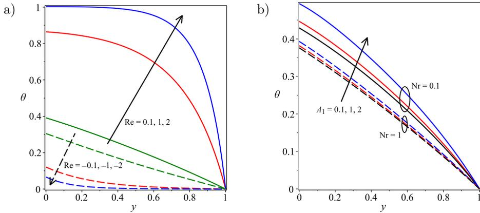
FIG. 9. Steady-state temperature profiles with increasing Re (a) and  $A_1$ , Nr (b).
