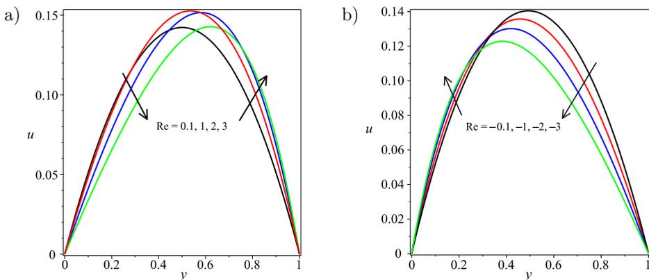
FIG. 6. Steady-state velocity profiles with increasing  $Re$ : a)  $Re > 0$ , b)  $Re < 0$ .
