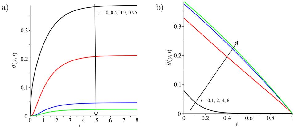
FIG. 4. Temperature profile across the channel: a) with increasing  $y$ , b) with increasing time  $t$ .
