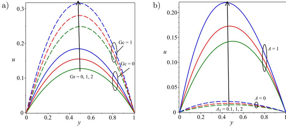
FIG. 7. Steady-state velocity profiles with increasing  $Gr$ ,  $Gc$  (a) and  $A_1$ ,  $A$  (b).
