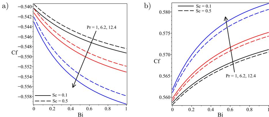
FIG. 13. Skin friction  $C_f$  vs. Biot number  $Bi$  with increasing  $Pr$  and  $Sc$ : a) at  $y = 0$ , b) at  $y = 1$ .
