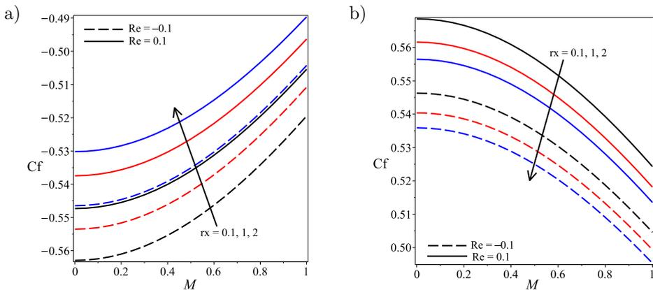
FIG. 15. Skin friction  $C_f$  vs. magnetic field parameter  $M$  with increasing  $rx$  and  $Re$ :
