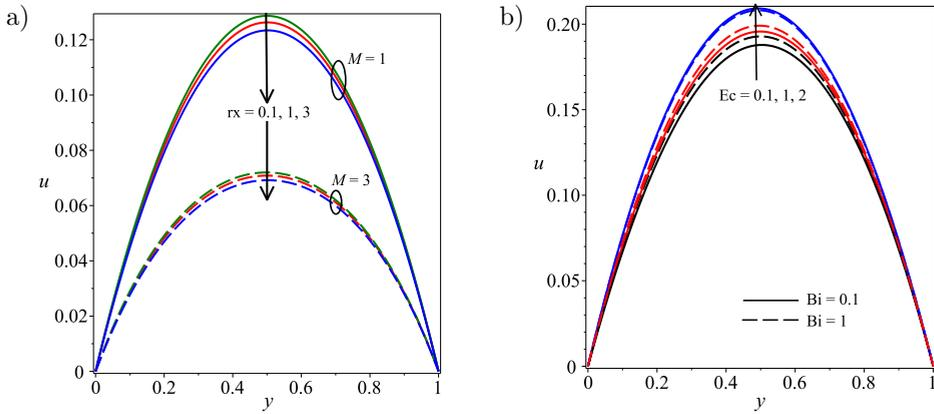
FIG. 8. Steady-state velocity profiles with increasing  $rx$ ,  $M$  (a) and  $Ec$ ,  $Bi$  (b).
