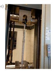
Fig. 8. a) Rope end with the original snap hook, b) sample mounted in the machine grips, c) sample view just before the break – snap hook was torn from the rope.
