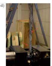
Fig. 7. a) Rope specimen prepared for the test on Z400 testing machine, b) sample placement in the machine, c) and d) rope specimen just before the break.
