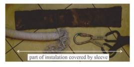
FIG. 1. Failed end of the rope along with a view of leg cuffs and a sleeve covering the rope end.
