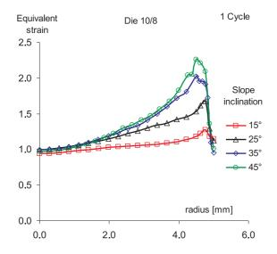
FIG. 7. Accumulated equivalent plastic strain versus the sample radius after one cycle of the CEC process, with  $d_0/d_m = 10/8$  and channel length a = 2 mm, for different inclination angles  $\alpha = 15^{\circ}, 25^{\circ}, 35^{\circ}, 45^{\circ}$  of conical parts of the die.
