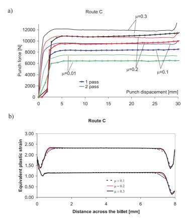
FIG. 16. Simulation results for ECAP Route C using Die I for different values  $\mu = 0.1$ , 0.2, 0.3 of the Coulomb friction coefficient, a) force acting on the punch versus the punch displacement, b) distribution of equivalent plastic strain across the billet.
