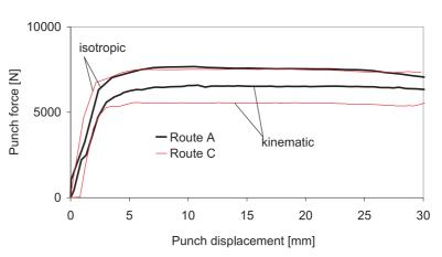
FIG. 19. Force acting on the punch versus the punch displacement during the second pass of ECAP, using Die II with negligible friction ( $\mu = 0.01$ ). The results are for routes A and C and for either isotropic or kinematic hardening.
