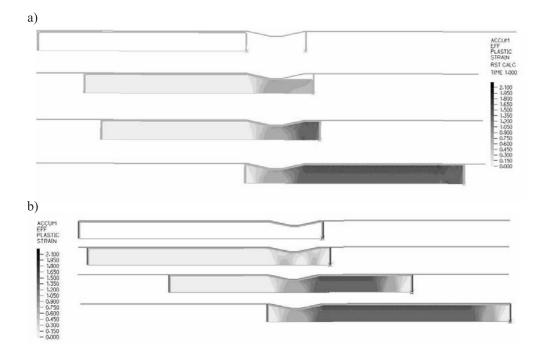
FIG. 5. Equivalent plastic strain field in the subsequent phases of the first pass in CEC process for two different sequences of calculation: a) initial position of the sample in the left chamber only, b) initial position of the sample covers the central channel.
