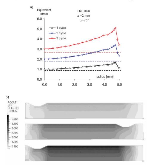
FIG. 10. Accumulated equivalent plastic strain after 1, 2 and 3 cycles of the CEC process, with  $d_0/d_m = 10/8$ , a = 2 mm and  $\alpha = 25^\circ$ ; a) distribution versus the sample radius, b) 2D distribution in the longitudinal cross-section.
