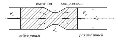
FIG. 1. Sketch of CEC deformation process.
