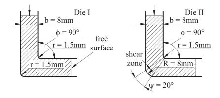
FIG. 14. Geometry of two ECAP dies used in numerical simulations.
