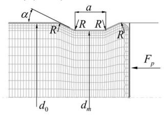
FIG. 2. Scheme of the finite element mesh and CEC channel geometry.
