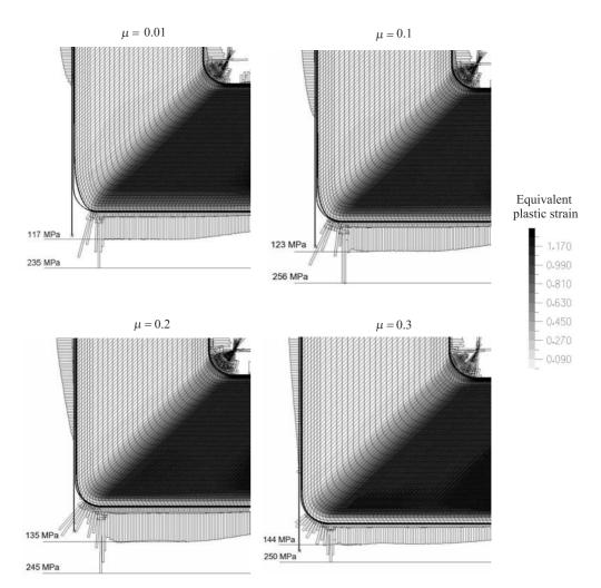
FIG. 15. Distribution of equivalent plastic strain and of surface tractions during the first pass through Die I, for different values  $\mu = 0.01, 0.1, 0.2, 0.3$  of the Coulomb friction coefficient. The development of the corner gap is dependent on the friction conditions.
