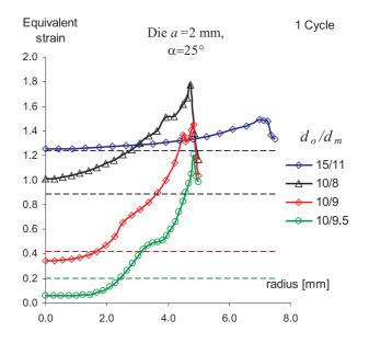
FIG. 6. Accumulated equivalent plastic strain versus the sample radius after one cycle of the CEC process, with different diameter ratios  $d_0/d_m = 15/11$ , 10/8, 10/9, 10/9.5. Channel length a = 2 mm, inclination angle of conical parts  $\alpha = 25^{\circ}$ , frictionless conditions.
