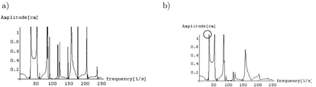
FIG. 6. Forced vibrations of the complex system for the stationary force and  $\gamma = 0.01$ ,  $\varepsilon = 1$ ;
