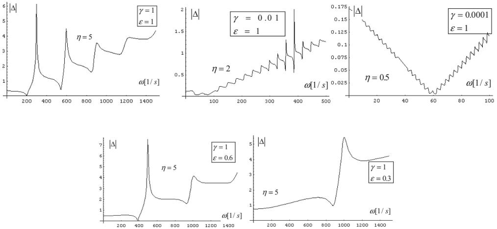
FIG. 2. Moduli of a complex determinant  $|\Delta|$  and values of complex eigenfrequencies  $\nu_{n_1 n_2} = i\eta_{n_1 n_2} \pm \omega_{n_1 n_2}$  of free vibrations for  $x = 0.6a, y = 0.6b, z = 0$  and  $n_1 = 1, n_2 = 1$ .
