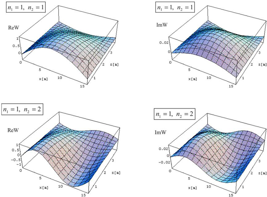
FIG. 3. Complex modes of free vibrations of the complex system with damping for  $n_1 = 1$ ,  $n_2 = 1$  and  $n_1 = 1$ ,  $n_2 = 2$ ; the elastic plate for  $z = 0$  and the visco-elastic inertial interlayer for  $0 < z < h$ .
