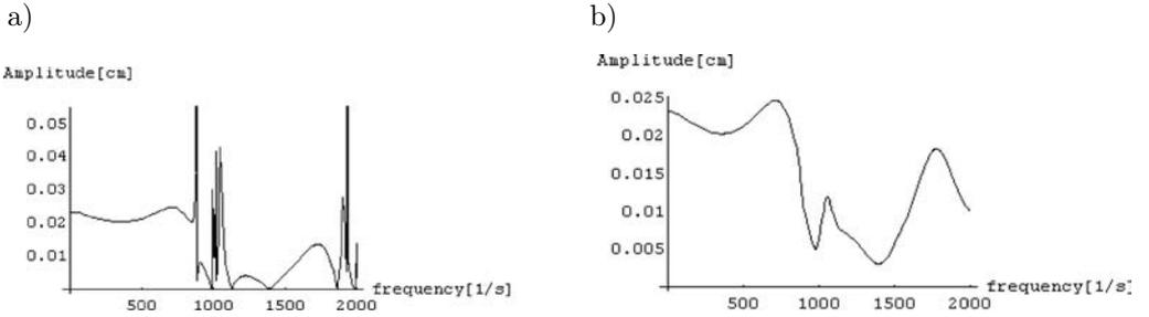
FIG. 9. Forced vibrations of the complex system for the stationary force and  $\gamma = 0$ ,  $\varepsilon = 0.3$ ;
