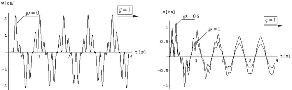
FIG. 11. Forced vibrations of the elastic and visco-elastic complex system for the mass moving with the speeds  $\zeta = 1$  and  $\gamma = 0.01$ ,  $\varepsilon = 1$ ,  $\varphi = \{0, 0.6, 1\}$ ,  $g = 1$ .
