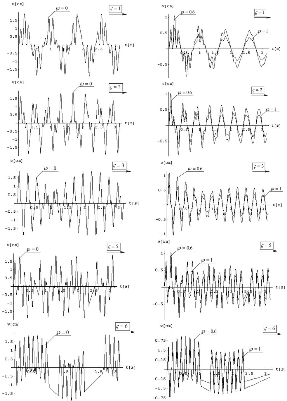
FIG. 10. Forced vibrations of the elastic and visco-elastic complex system for the moving mass with the speeds  $\zeta = \{1, 2, 3, 5, 6\}$  for  $\gamma = 1$ ,  $\varepsilon = 1$ ,  $\varphi = \{0, 0.6, 1\}$ ,  $g = 1$ .
