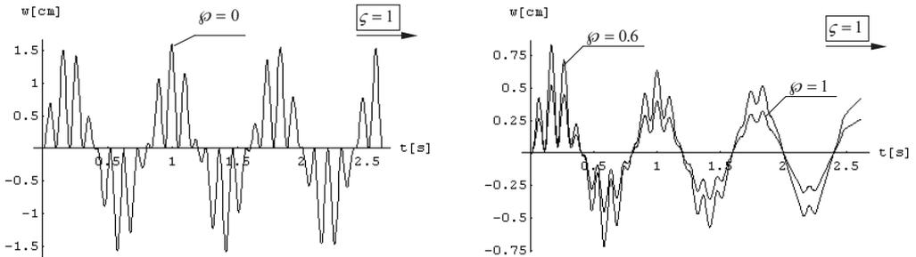
FIG. 12. Forced vibrations of the elastic and visco-elastic complex system for the mass moving with the speeds  $\zeta = 1$  and  $\gamma = 1$ ,  $\varepsilon = 0.03$ ,  $\varphi = \{0, 0.6, 1\}$ ,  $g = 1$ .
