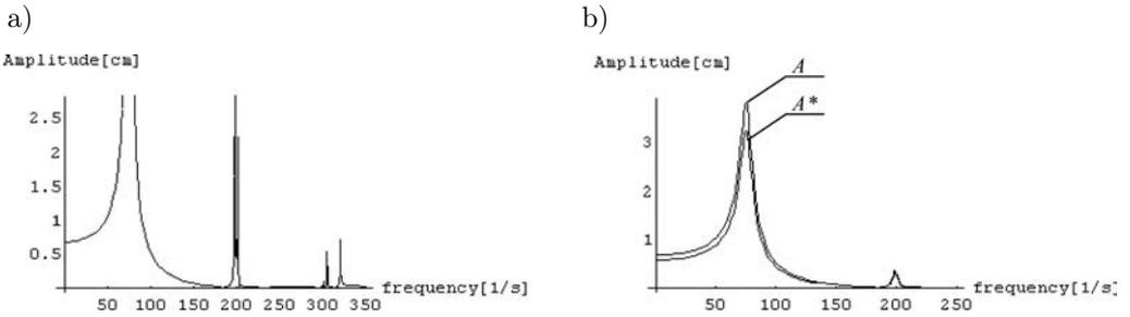
FIG. 5. Forced vibrations of the complex system for the stationary force and  $\gamma = 1$ ,  $\varepsilon = 1$ ;
