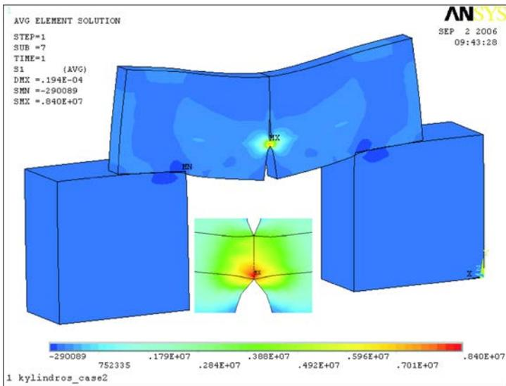
FIG. 4. The distribution of the 1st (maximum) principal stress in the restored architrave. The embedded figure shows a detail of the central section around the titanium bar.
