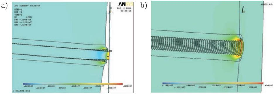
FIG. 10. A detailed view of the distribution of the 2-nd principal stress around the central cross-section area of the titanium bar (a) and of the marble (b).
