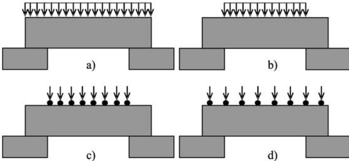
FIG. 3. The four loading cases studied numerically.
