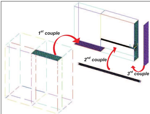
FIG. 8. Identification of the contact elements created for the model.
