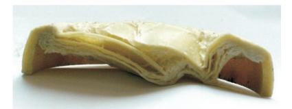
FIG. 12. Cross-section of the destroyed sphere shows delamination of the plays.
