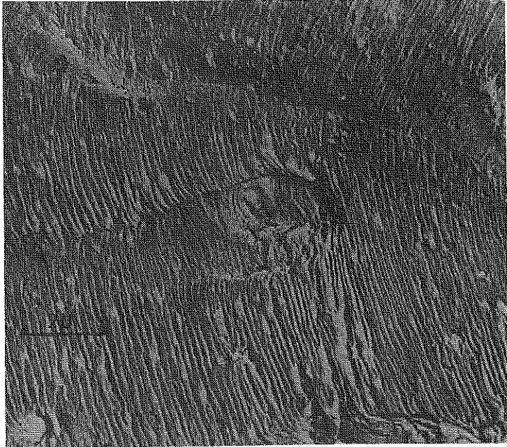
FIG. 16. Fatigue striations in Al-Cu-Mg alloy (from [61]).
