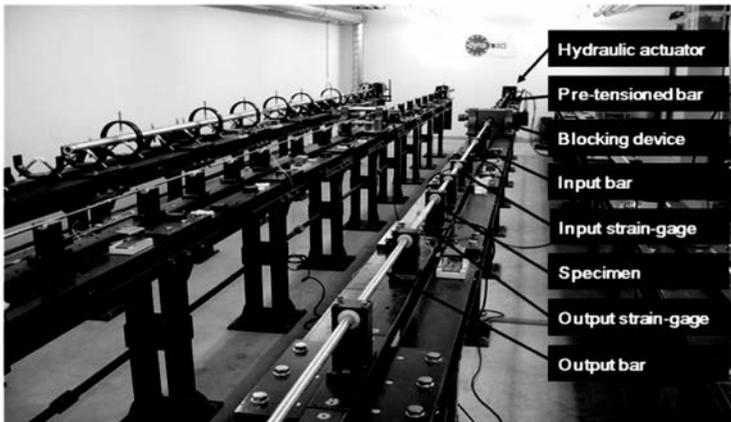
FIG. 3. Dynamic direct tensile testing set-up.
