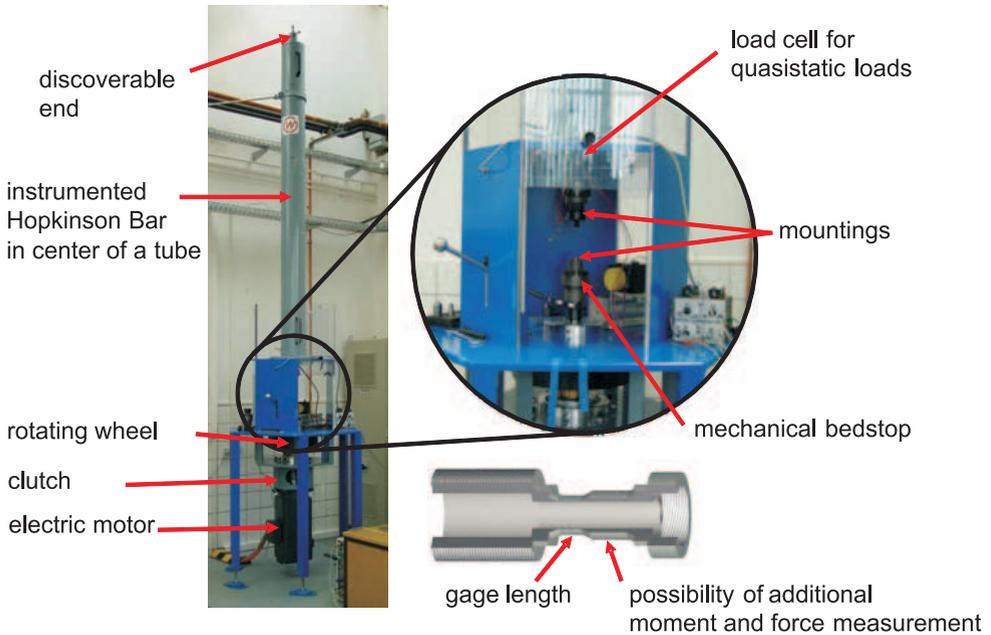
FIG. 3. Combined static and impact dynamic universal testing machine.
