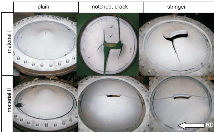
FIG. 6. Failure characteristics for two different materials at different pre-treatment states after biaxial testing.
