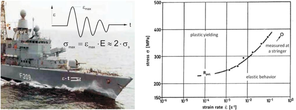
FIG. 1. Dynamic loading of a canon shooting on a Navy ship structure.
