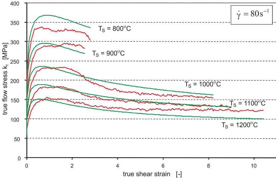
FIG. 4. Flow stress evolution of a low alloyed steel at high strains, high shear rate and high temperatures: comparison of experimental data and modeled data using the Hensel-Spittel approach [5].
