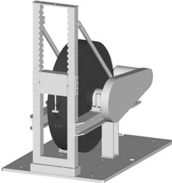
FIG. 8. Rotating wheel device of Nordmetall GmbH with a high amount of stored energy, by a 10 t flywheel ( $\varnothing 2$  m) for dynamic component testing of engineering materials.
