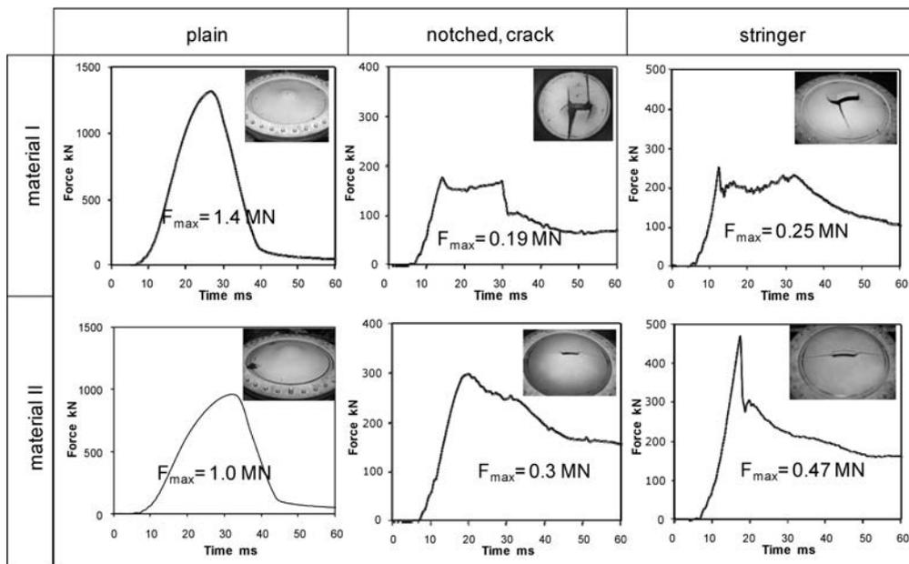
FIG. 7. Force-time behavior of two different materials with different stress-states at dynamic biaxial loading.
