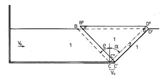
Fig. 17. The kinematically admissible solution at a certain stage of the rigid wall pressure process (for the Tresca yield criterion material) - first step.
