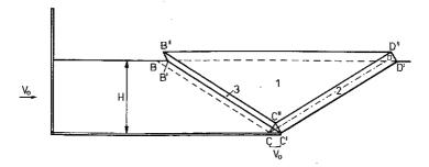
Fig. 8. The kinematically admissible solution at a certain stage of the rigid wall pressure process (first step).
