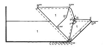
Fig. 20. The kinematically admissible solution at a certain stage of the rigid wall pressure process (for the Tresca yield criterion material) – after advanced tool displacement.
