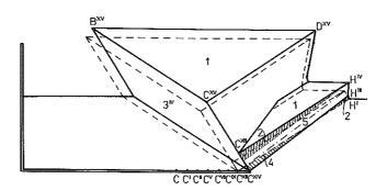
Fig. 12. The kinematically admissible solution at a certain stage of the rigid wall pressure process (after advanced tool displacement).
