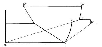
Fig. 14. The kinematically admissible solution for the tool rotation process.
