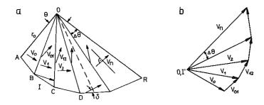
Fig. 16. The kinematically admissible mechanism for the stiff wall rotation process.
