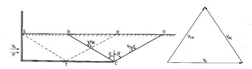
Fig. 2. The rigid wall (shaped similar to the bucket of a loading machine) pressure problem and its kinematically admissible solution.
