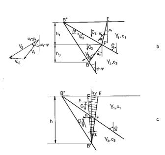
Fig. 13. Different mechanisms for the soil wedge sliding process.
