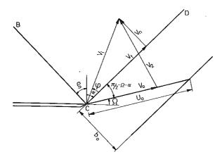
Fig. 7. The material velocity on the tool edge.
