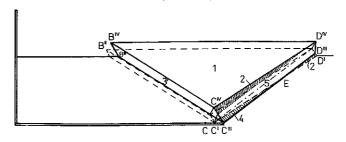
Fig. 9. The kinematically admissible solution at a certain stage of the rigid wall pressue process.
