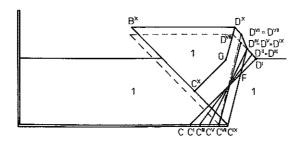
Fig. 19. The kinematically admissible solution at a certain stage of the rigid wall pressure process (for the Tresca yield criterion material) – advanced tool displacement.
