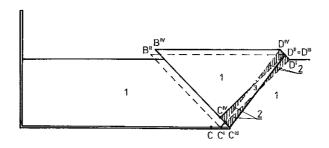
Fig. 18. The kinematically admissible solution at a certain stage of the rigid wall pressure process (for the Tresca yield criterion material).
