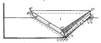
Fig. 10. The kinematically admissible solution at a certain stage of the rigid wall pressure process.
