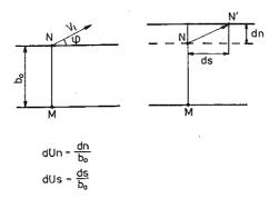
Fig. 5. Dilatation and shear processes on a slip line in the case of the associated flow rule assumption.
