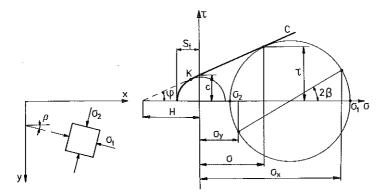
Fig. 1. The modified Coulomb-Mohr yield criterion for plane strain conditions in the  $\sigma - \tau$  axes.
