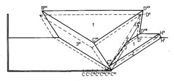
Fig. 11. The kinematically admissible solution at a certain stage of the rigid wall pressure process (advanced tool displacement).
