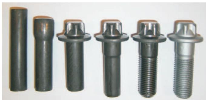
FIG. 2. Sequence of cold forming of fastener.
