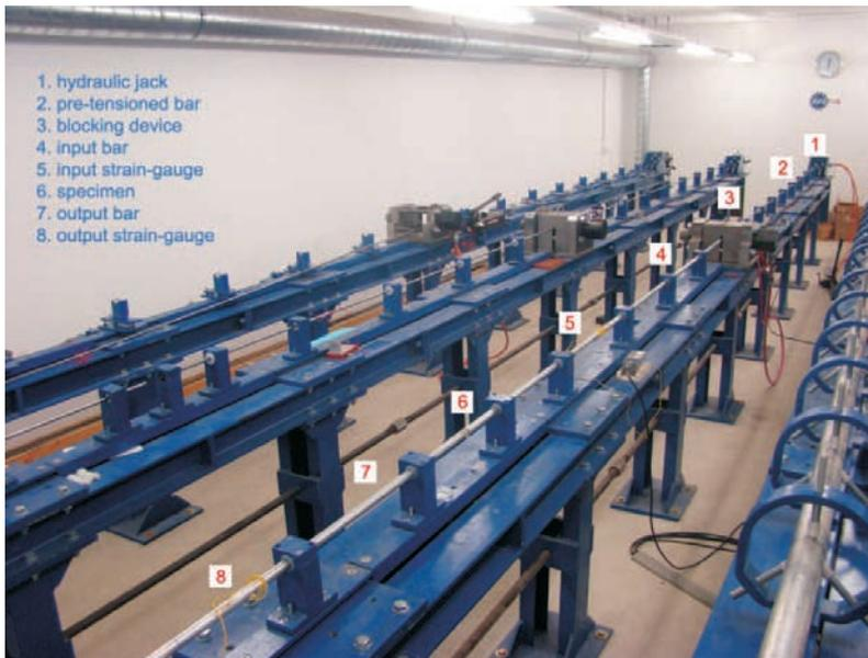
FIG. 3. High strain-rate tensile tests on specimen  $\varnothing = 20$  mm.
