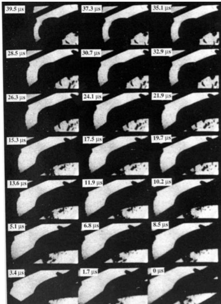
FIG. 10. Selected frames from the high-speed photographic sequence of the impact of a 5 mm thick RHA steel plate at  $60^\circ$  on a round-nosed tungsten alloy rod at  $645\ \text{m s}^{-1}$ . Note that in this sequence the time at which impact occurred is not known, so the first frame (bottom right) is set as time zero.
