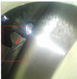
FIG. 10. Root flaw of the planet gear.
