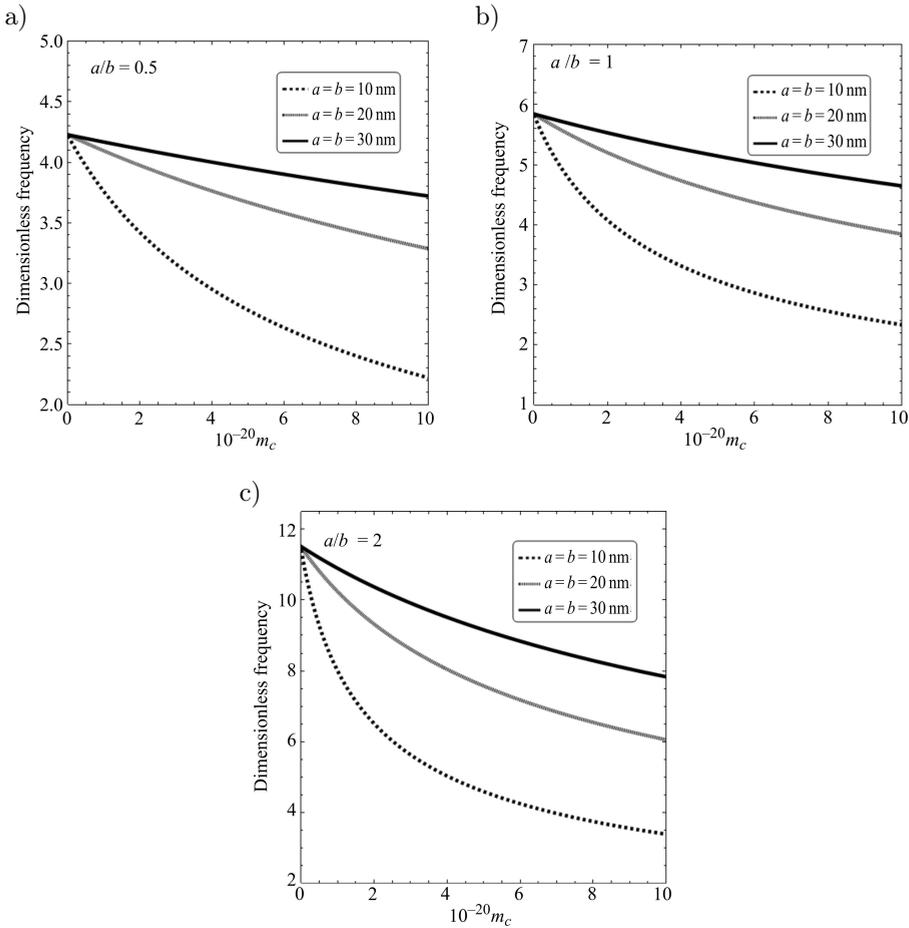
FIG. 7. Dimensionless frequency of graphene sheet *versus* nanoparticle mass for various aspect ratios ( $\mu = 0.2$ ,  $\lambda = 0.1$ ,  $K_w = 25$ ,  $K_p = 5$ ).
