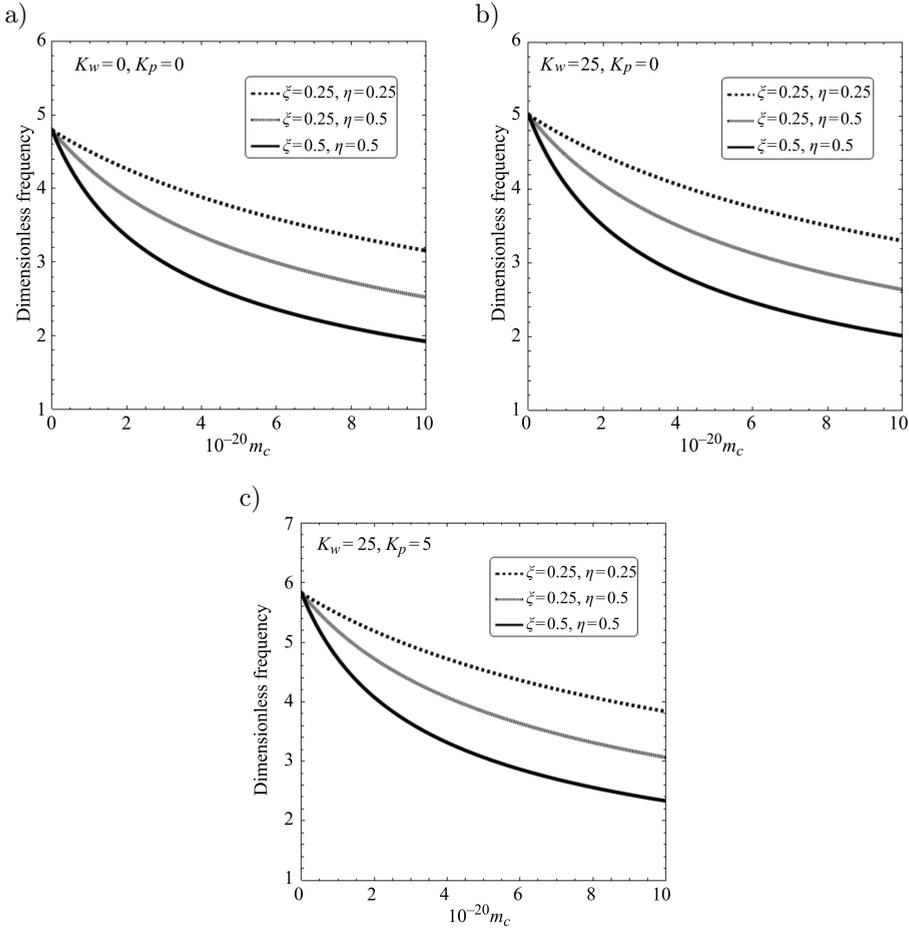
FIG. 6. Dimensionless frequency of graphene sheet *versus* nanoparticle mass for various foundation parameters and nanoparticle location ( $\mu = 0.2, \lambda = 0.1$ ).
