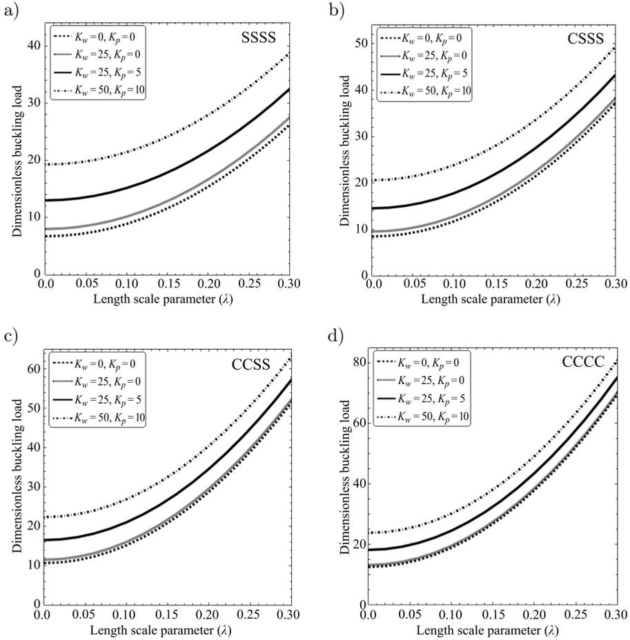
FIG. 5. Variation of the dimensionless buckling load *versus* length scale parameter for different foundation parameters and boundary conditions ( $\mu = 0.2, \lambda = 0.1, \Delta T = 50, \Delta C = 0.1$ ).
