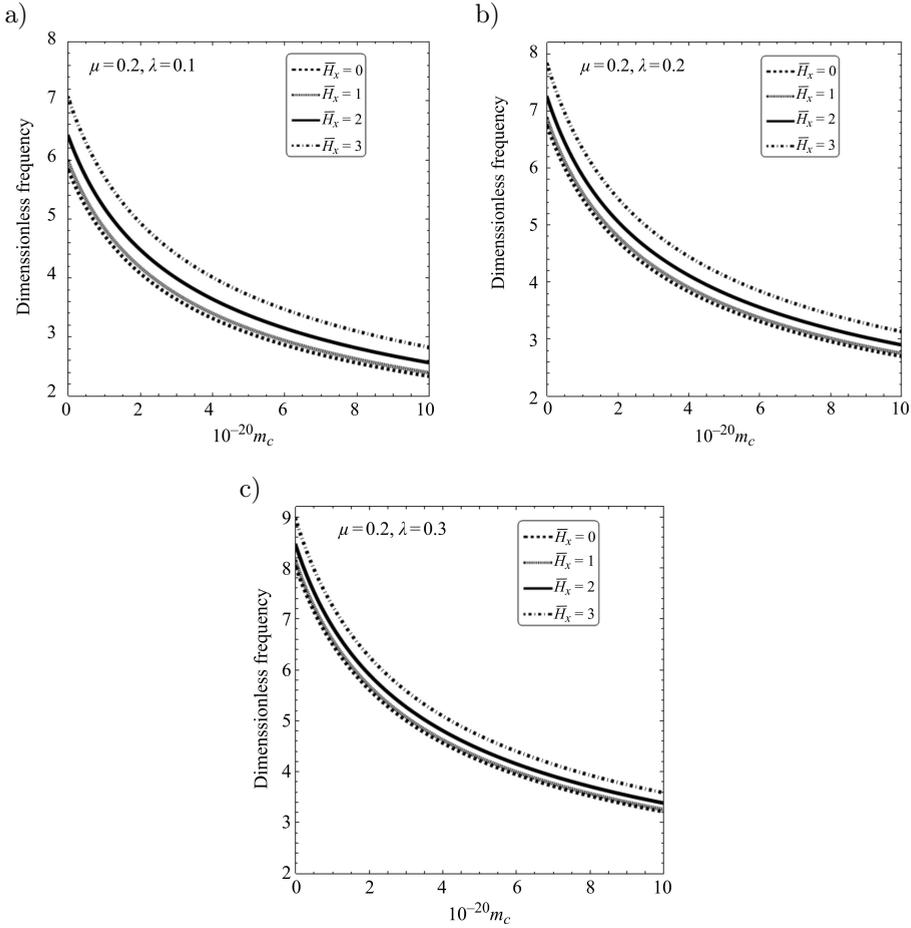
FIG. 8. Dimensionless frequency of graphene sheet *versus* nanoparticle mass for various magnetic fields.
