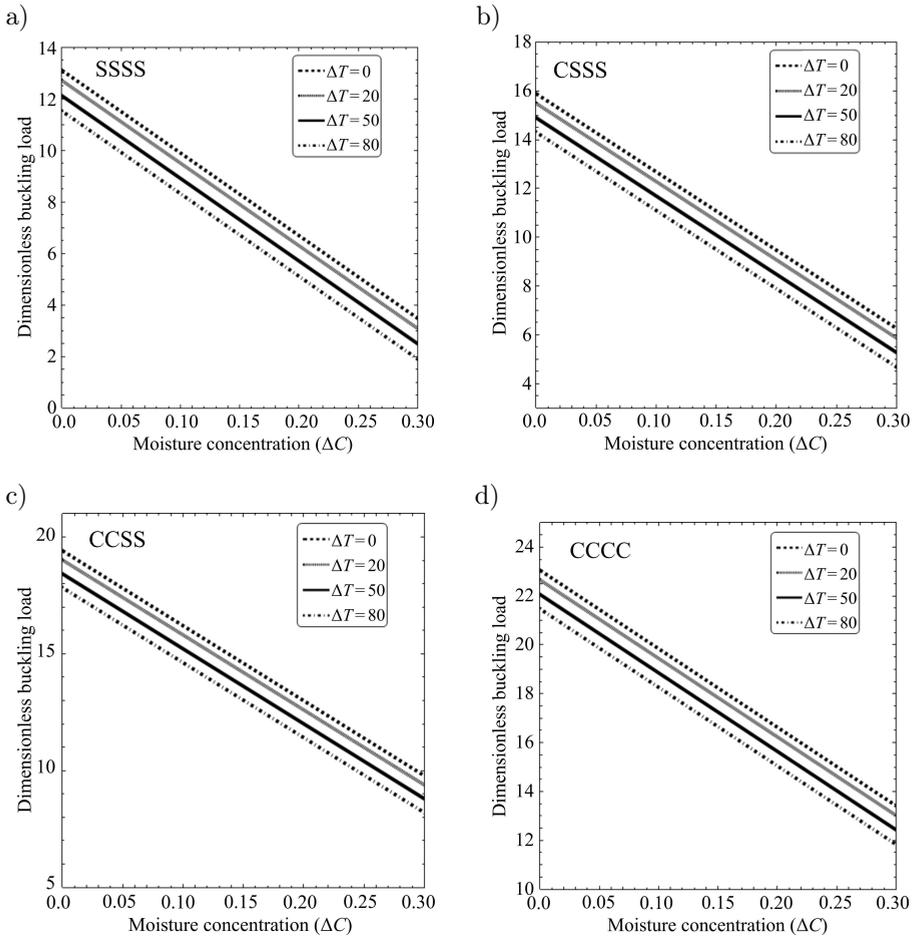
FIG. 4. Variation of the dimensionless buckling load *versus* moisture rise for different temperature changes and boundary conditions ( $\mu = 0.2, \lambda = 0.1$ ).
