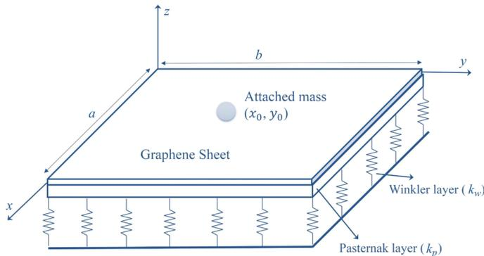
FIG. 1. Configuration of graphene sheet resting on an elastic substrate.
