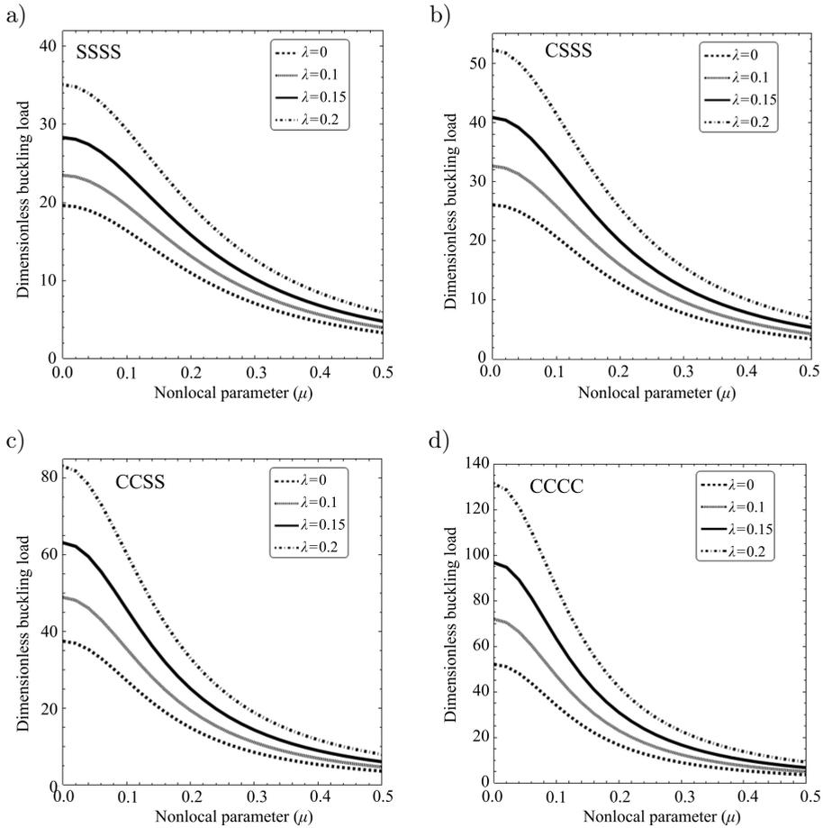
FIG. 3. Variation of the dimensionless buckling load *versus* nonlocal parameter for different length scale parameters and boundary conditions.
