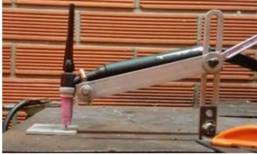
FIG. 1. Torch support for keeping constant the arc length.
