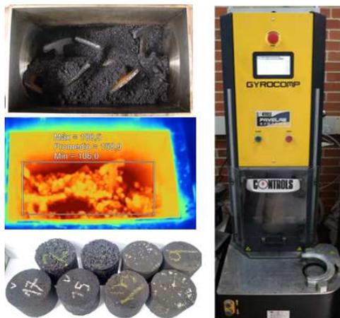
FIG. 4. Manufacture of asphalt mixtures.
