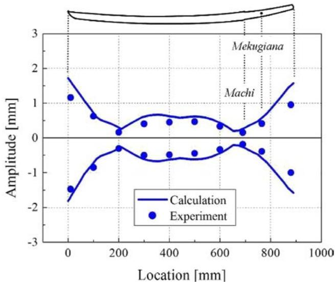
FIG. 12. Comparison between the measured and simulated amplitudes (impact position of 100 mm).
