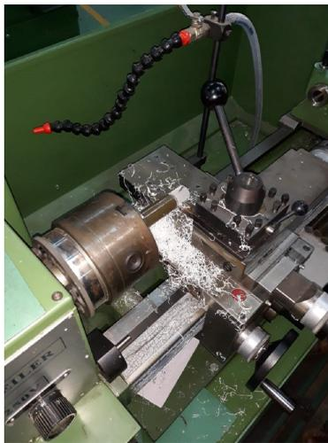
FIG. 2. Machining of the composite sample.
