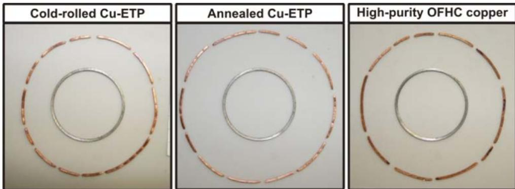
FIG. 6. View of recovered fragments generated from different sorts of copper rings.
