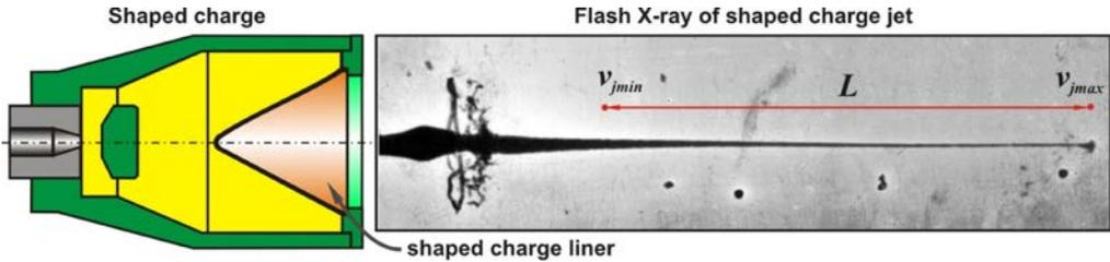
FIG. 1. Typical shaped charge configuration and rentgenogram of shaped charge jet.
