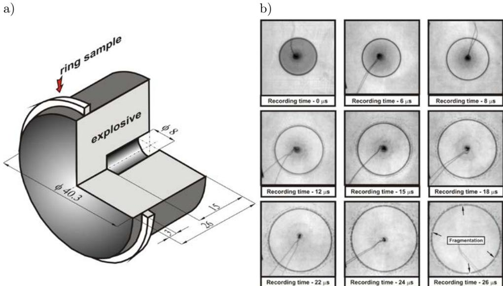
FIG. 2. Scheme of the experimental set-up driving explosively the ring sample (a) and radiographs of explosively expanding rings made of copper sinter (b) [9].
