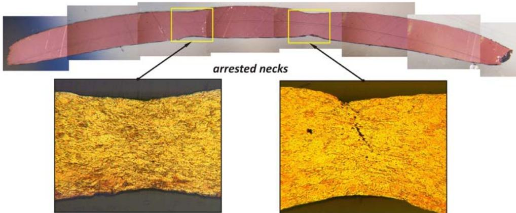
FIG. 7. View of the annealed copper ring fragment and the structures of the arrested necks arisen into ring fragment.
