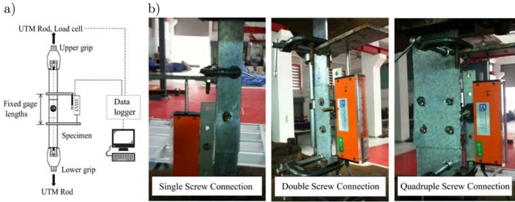
FIG. 2. Screw connection test setup: a) test apparatus, b) test specimen.
