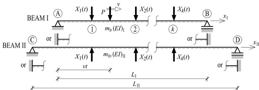
FIG. 2. Two single-span beams subjected to moving force and redundant forces.
