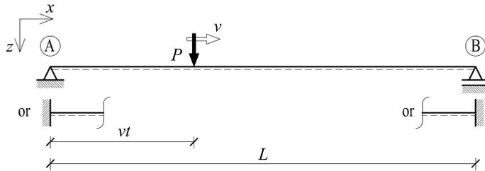
FIG. 3. Single-span beam subjected to a moving point force.
