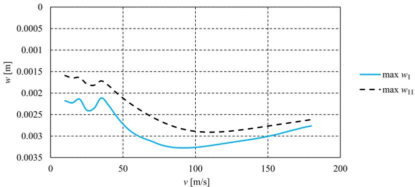
FIG. 8. Maximum dynamic deflection throughout the upper and the lower beam *versus* different force movement velocities.
