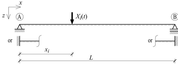
FIG. 4. Single-span beam subjected to a concentrated time-varying force.
