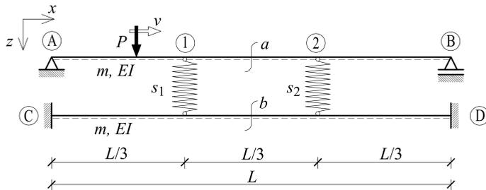
FIG. 5. Double-beam system with two elastic restraints loaded with moving point force.
