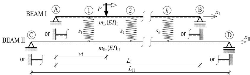
FIG. 1. Double-beam system with intermediate elastic restraints subjected to a moving force.
