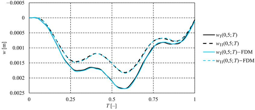
FIG. 6. Dynamic deflection of the middle of the upper and the lower beam.
