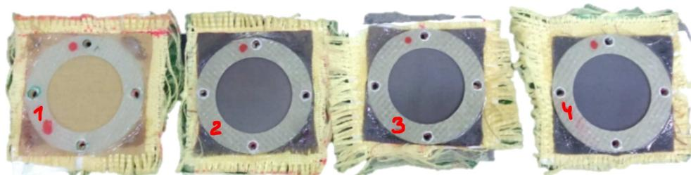
FIG. 14. Samples for gas impact resistance test.
