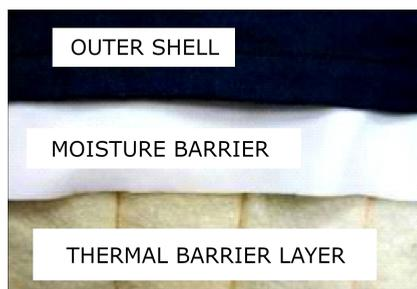
FIG. 1. Three-layered arrangement of materials.
