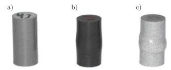
FIG. 12. View of specimens after fatigue tests: a) Chester Metal Rapid, b) Unirep 1, and c) Belzona 1221.
