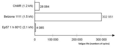
FIG. 15. Comparison of the relative shear fatigue life of adhesive composites (the maximum load of fatigue cycle was  $\sim 0.66F_n$ ).
