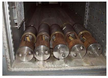
FIG. 4. The view of devices together with the mounted and loaded specimens used to determine long-term strength of adhesive joints.
