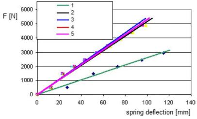
FIG. 5. Characteristics of the springs used in devices with the imposed loads.
