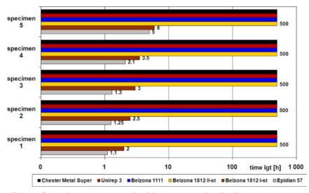
FIG. 8. Static long-term strength of lap joints made of adhesive composites (loaded with a power of 60%  $F_n$  and at a temperature of 60°C).
