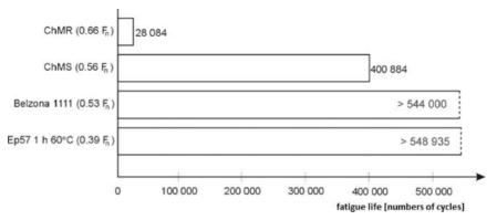
FIG. 14. Comparison of the absolute shear fatigue life of adhesive composites (the maximum load of a fatigue cycle was 1.3 kN for all adhesives).
