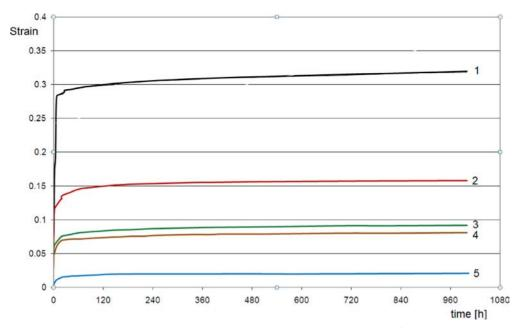
FIG. 7. Creep curves of the adhesive composites in the temperature of 60°C with load causing normal stresses of 30 MPa in the examined specimens (1 – Epidian 57, 2 – Chester Metal Super, 3 – Belzona 1111, 4 – Unirep 3, 5 – Belzona 1812 – II st.).
