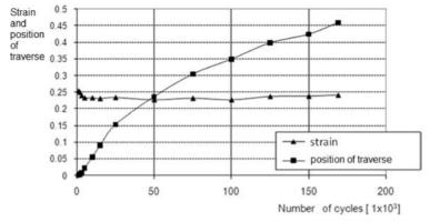
FIG. 16. Change of specimen's strain and position of the traverse (change in specimen's height) during fatigue tests of Belzona 1111 adhesive composite.
