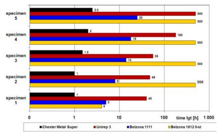
FIG. 9. Static long-term strength of lap joints made of the adhesive composites (load with power of 60%  $F_n$  and temperature of 100°C).
