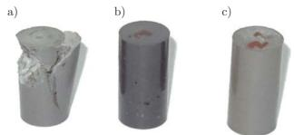
FIG. 11. View of specimens after fatigue tests: a) Chester Metal Super, b) Unirep 3, c) Belzona 1111.
