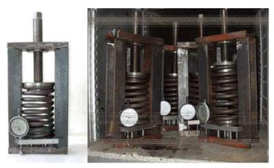
FIG. 1. View of the device used to determine creep curves with mounted and loaded specimens.
