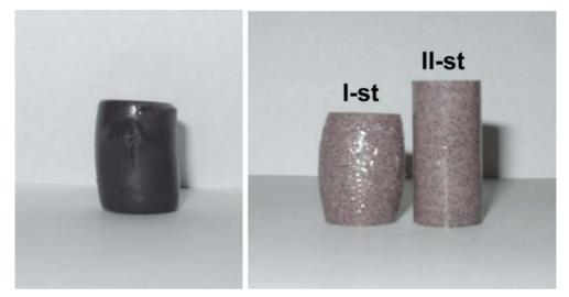
FIG. 6. Unirep 1 and Belzona 1812 (after single-stage stage curing) adhesive composites after a few minutes from the moment of 30 MPa load at a temperature of  $60^{\circ}$ C.
