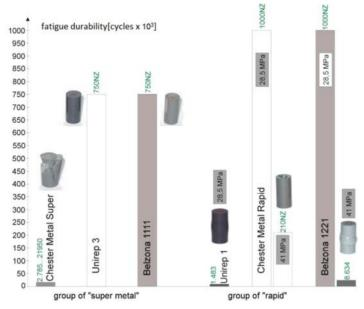
FIG. 13. Fatigue life of the adhesive composites examined (NZ – specimen was not damaged during the test).
