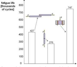
FIG. 10. Influence of the specimen's shape and load method on the average fatigue life of joints made of epoxy adhesive Epidian 57/Z1 [5].
