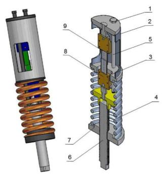
FIG. 3. The device used to determine static long-term strength of adhesive joints: 1, 3 - covers;
