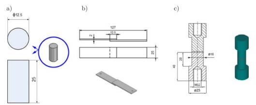
FIG. 2. Shape and dimensions of specimens used to determine properties of adhesive composites.
