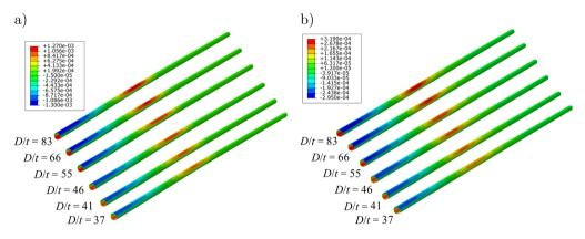
FIG. 6. Axial strain of the pipeline under different radius-thickness ratios: a) pipeline-1, b) pipeline-2.
