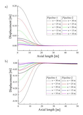
FIG. 14. Displacement of the pipeline under different widths: a) horizontal displacement (x-direction), b) vertical displacement (z-direction).
