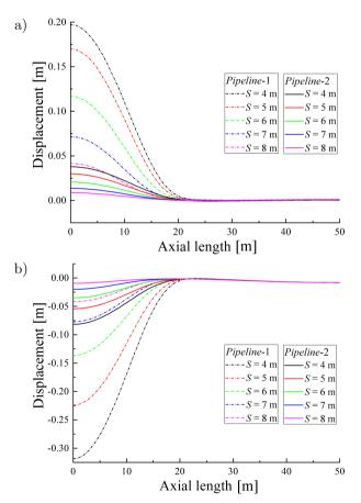
FIG. 11. Displacement of the pipeline under different distances: a) horizontal displacement (x-direction), b) vertical displacement (z-direction).
