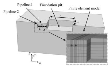
FIG. 1. Schematic diagram of foundation pit.
