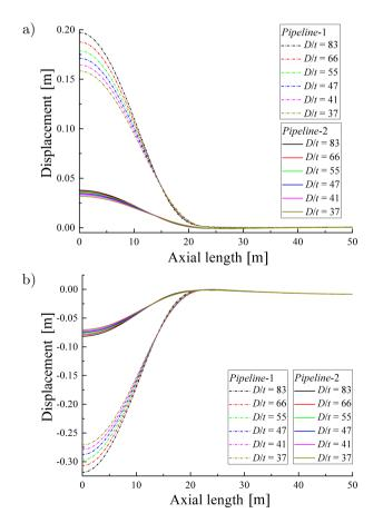
FIG. 8. Displacement of the pipeline under different radius-thickness ratios: a) horizontal displacement (x-direction), b) vertical displacement (z-direction).
