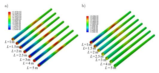
FIG. 4. Axial strain of the pipeline under different parallel distances: a) pipeline-1, b) pipeline-2.
