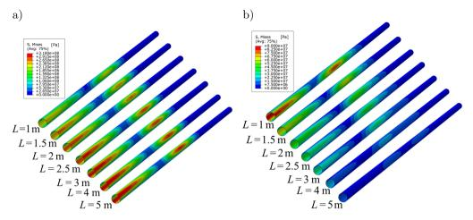
FIG. 2. Stress of the pipeline under different parallel distances: a) pipeline-1, b) pipeline-2.
