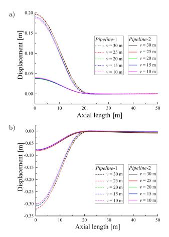
FIG. 16. Displacement under different lengths: a) horizontal displacement (x-direction), b) vertical displacement (z-direction).
