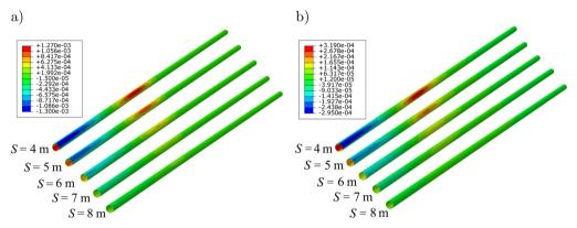
FIG. 9. Axial strain of the pipeline under different distances: a) pipeline-1, b) pipeline-2.
