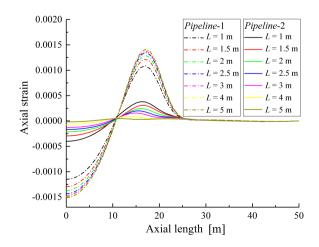
FIG. 5. Axial strain curves of the upper surface under different parallel distances.
