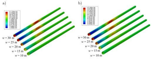
FIG. 12. Axial strain of the pipeline under different widths: a) pipeline-1, b) pipeline-2.
