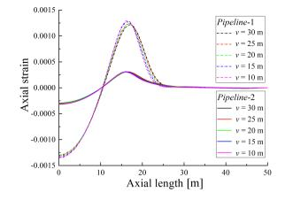
FIG. 15. Axial strain curves of the upper surface under different lengths.
