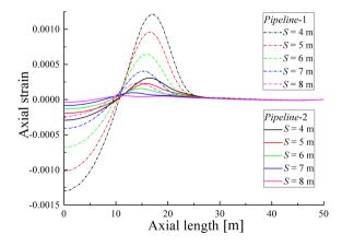
FIG. 10. Axial strain curves of the upper surface under different distances.
