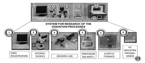
FIG. 4. Research corrosion stand.
