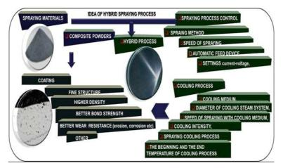
FIG. 3. Idea of hybrid spraying process.
