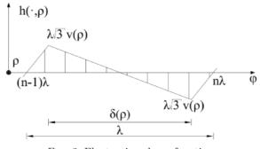
FIG. 3. Fluctuation shape function.
