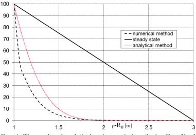
FIG. 4. The results of analytical and numerical method – Case No. I after t = 1 [h]. A diagram of averaged temperature.
