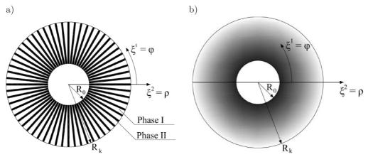
FIG. 1. Structure of two-phase functionally graded composites on a) micro- and b) macro-scale.
