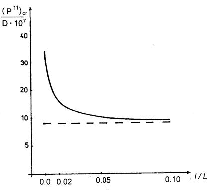
FIG. 3. The smallest value of a critical forces  $(P^{11})_{cr}$  for a long rectangular plate resting on the Winkler elastic foundation versus ratio l/L, for a microstructural and a orthotropic models.
