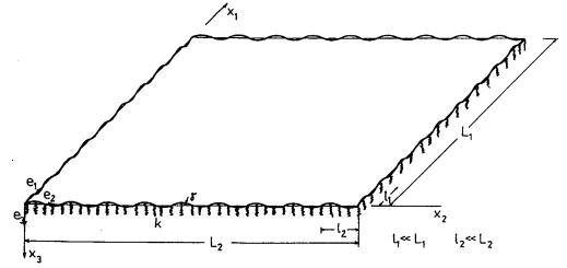
FIG. 1. A scheme of the wrinkled plate on an elastic foundation.
