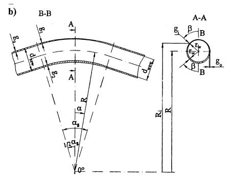
FIG. 1. a, b. Geometrical quantities in the pipe bending description.
