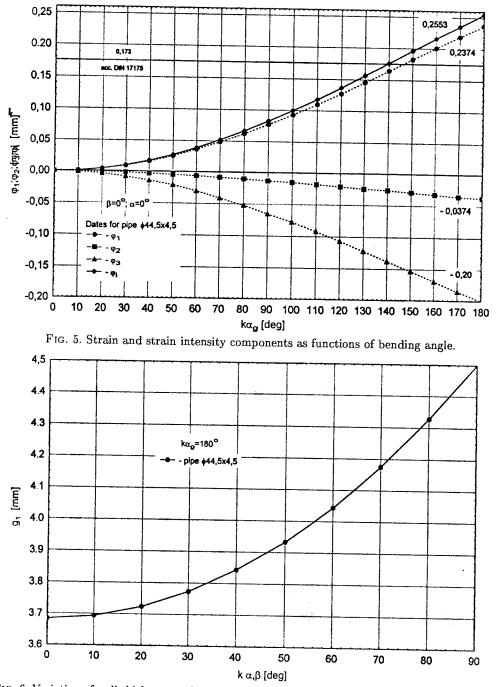
FIG. 6. Variation of wall thickness at the principal plane of bending and at planes perpendicular to it.
