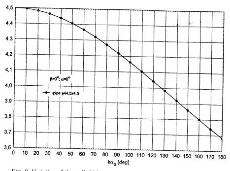
FIG. 2. Variation of the wall thickness at the apex point of the elongated area.
