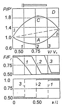
FIG. 3. Results of optimization of the cantilever beam with respect to the maximum and minimum of the first natural frequency.
