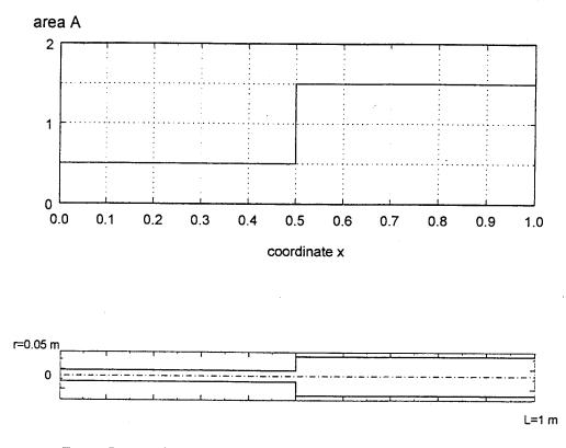
FIG. 7. Results of minimization of  $\mu^*$  for the cantilever beam for  $\beta_0 = 0.6$ .
