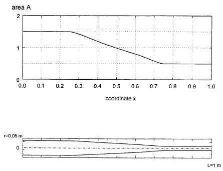
FIG. 5. Results of monocriterion optimization of the beam with respect to the maximum of  $\mu^*$ . The nondimensional area A of cross-section of the beam versus the nondimensional coordinate x and the shape of the cantilever beam for  $\beta_0 = 0.2$ .
