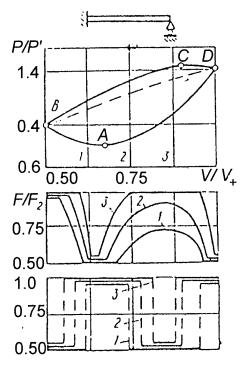
FIG. 2. Results of optimization of simply supported-fixed beam with respect to the maximum and minimum of the first natural frequency.
