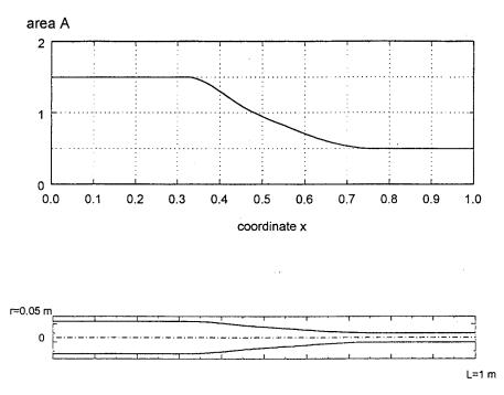
FIG. 6. Results of monocriterion optimization of the beam with respect to the maximum of  $\mu^*$ . The nondimensional area A of cross-section of the beam versus the nondimensional coordinate x and the shape of the cantilever beam for  $\beta_0 = 0.6$ .
