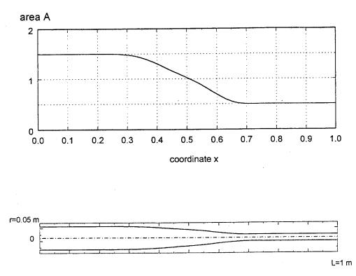
FIG. 4. Results of monocriterion optimization of the beam with respect to the maximum of  $\mu^*$ . The nondimensional area A of cross-section of the beam versus the nondimensional coordinate x and the shape of the cantilever beam for  $\beta_0 = 0$ .
