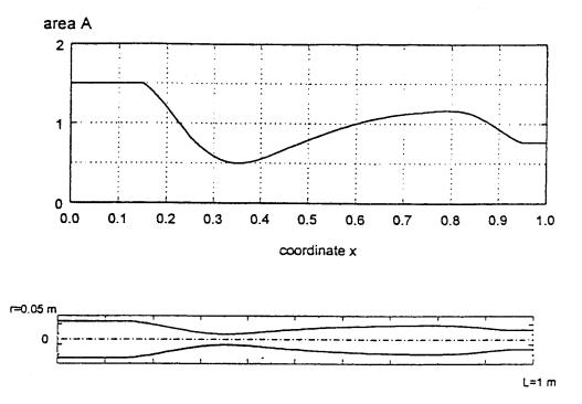
FIG. 8. Results of multicriterial optimization of the beam with respect to the maximum of  $\mu^*$ . The nondimensional area A of cross-section of the beam versus the nondimensional coordinate x and the shape of simply supported-fixed beam for  $\beta_0 = 0$ .
