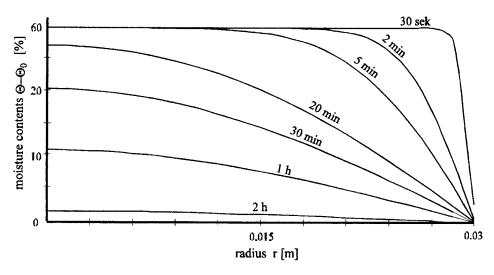
FIG. 4. Moisture contents distribution in the sphere.
