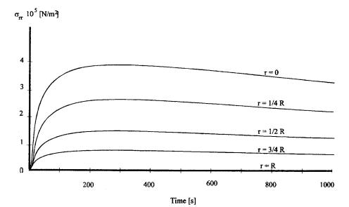
FIG. 5. Radial stresses as a function of time for different radii.
