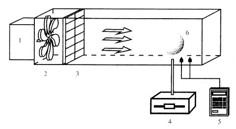
FIG. 3. Experimental equipment. 1 – electric heater, 2 – blower, 3 – heater and wire mesh, 4 – electronic balance, 5 – thermometer, 6 – clay sample.
